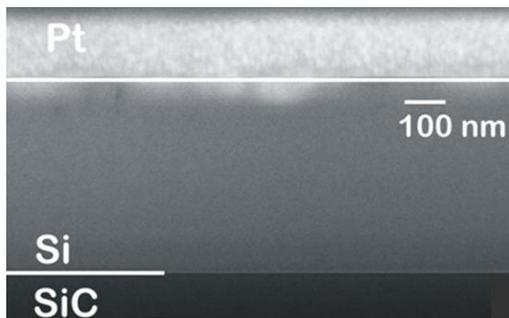
Fig. 2: SEM image showing cross-section of the Si/SiC heterojunction structure.
