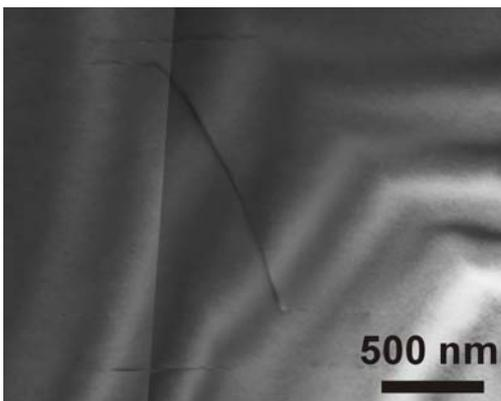
Fig. 4: A TEM image from the layer grown on C face 6H-SiC substrate using mixture of Si and Al as a solvent. It reveals the enhanced formation of dislocations in the near substrate /layer interface region.
