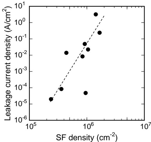
Fig. 4: Change in leakage current of a pn diode as a function of SF density. An one order of magnitude increase in the SF density enhances the leakage current five orders of magnitude.
