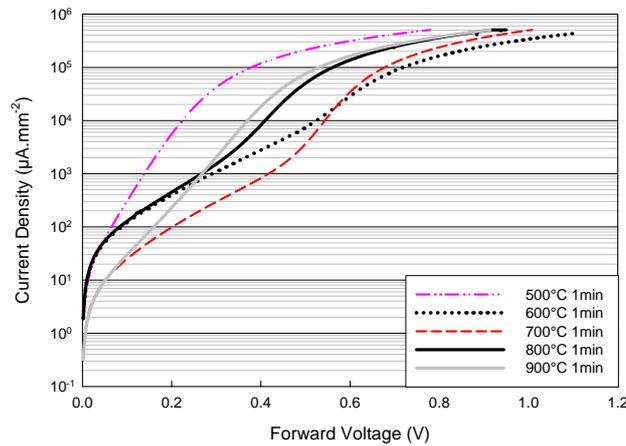
Fig. 3: J(V) forward characteristics represented for 0.17 mm<sup>2</sup> platinum anodes annealed between 500 °C and 900 °C.
