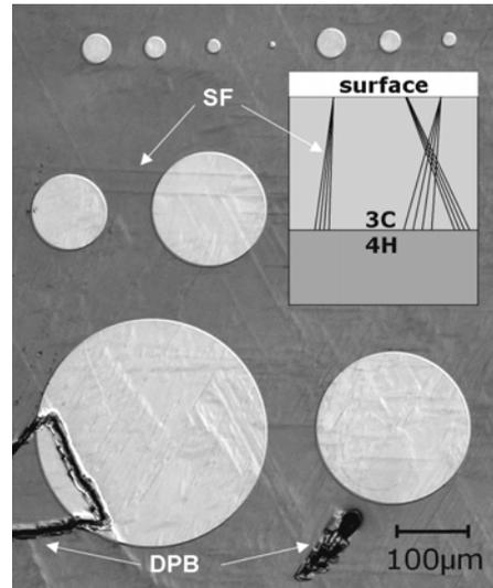
Fig. 2: Optical image showing possible SF and DPB defects on the diodes. Cross-section drawing illustrates SF originating from interface to surface.
