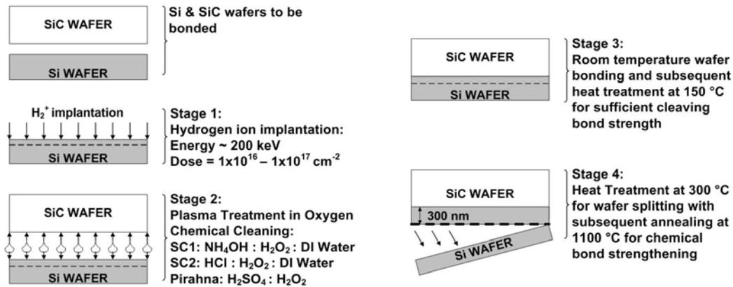
Fig. 1: Summary of the Si/SiC wafer bonding process undertaken in this work.
