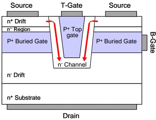
Fig. 1: Schematic drawing of all-epitaxial SiC double-gate trench JFET (DGTJFET).
