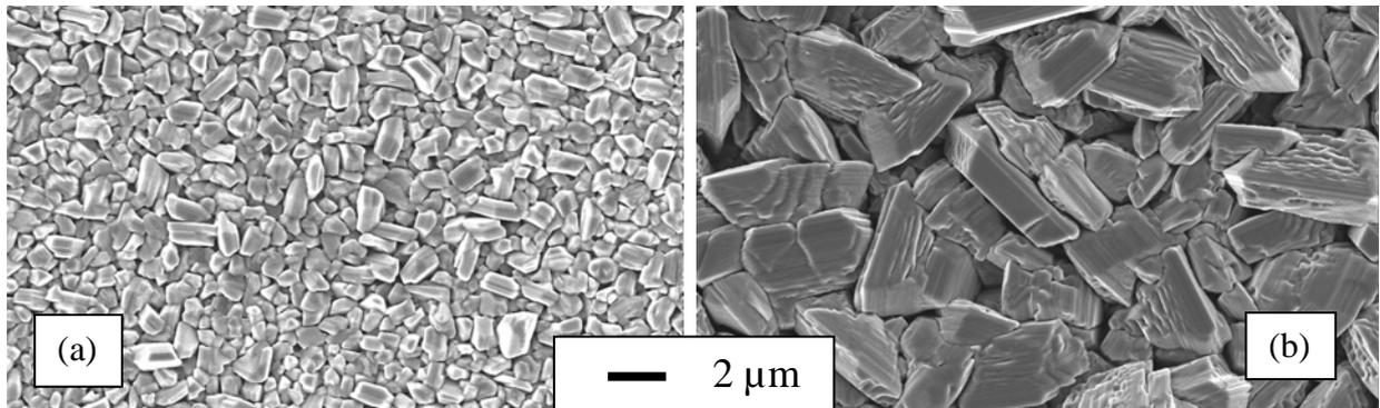
Fig.2: SEM micrographs of poly 3C-SiC films with thicknesses: (a) 1.5  $\mu\text{m}$  and (b) 15  $\mu\text{m}$ .
