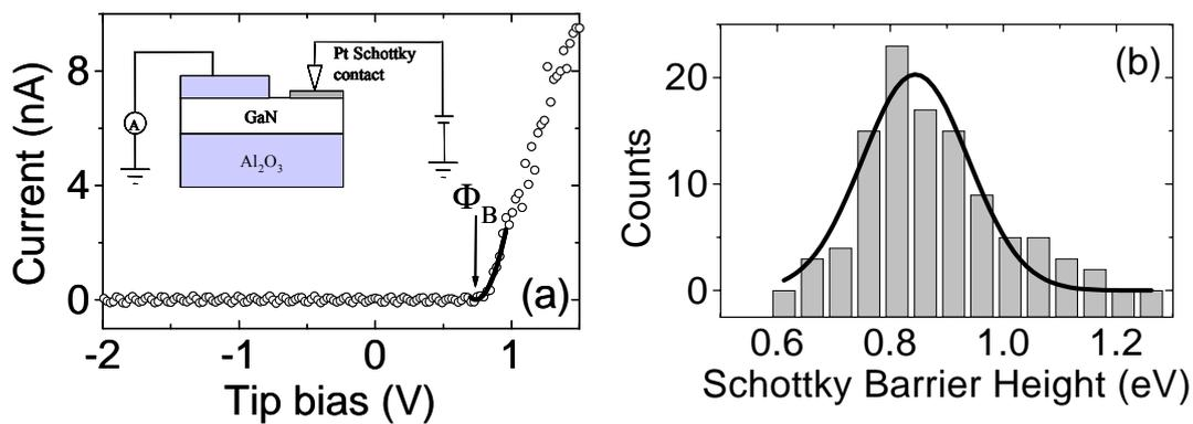
Fig. 2: (a) Local I-V curve measured placing the nanometric C-AFM tip on a thin Pt layer deposited on GaN; the estimated value of the local SB height is indicated. (b) Histogram of the barrier height distribution for the laterally inhomogeneous Pt/GaN contact.
