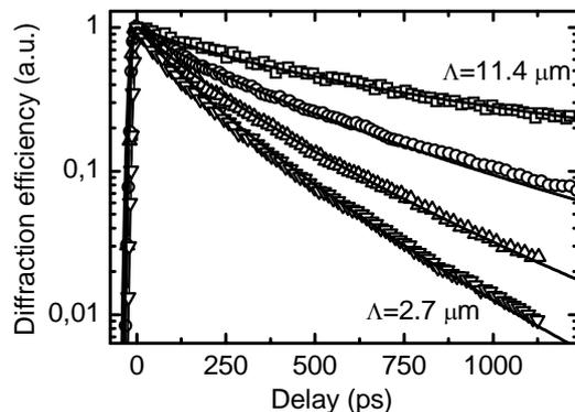
Fig. 1: FCG kinetics in HVPE GaN at different grating periods  $\Lambda$  (2.7, 3.2, 4.3, and  $11.4 \mu\text{m}$ ): experimental data (points) and modelling, using  $B = 2 \times 10^{-11} \text{ cm}^{-3}/\text{s}$  value and  $D = D_0(1 + N/N_0)$  dependence with  $N_0 = 2 \times 10^{19} \text{ cm}^{-3}$ . Excitation density  $I = 2.7 \text{ mJ}/\text{cm}^2$ .
