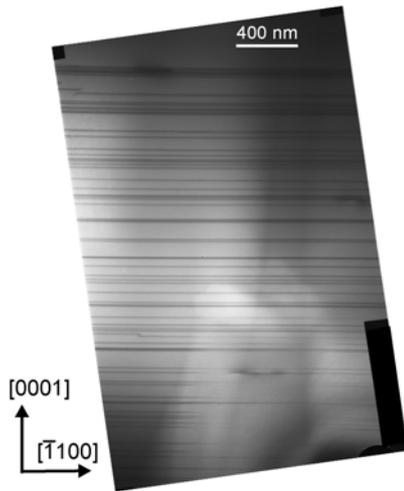
Fig. 1: A TEM micrograph, showing the relatively high SF density in the layers grown on the Si face substrates with pure Si used as a solvent.
