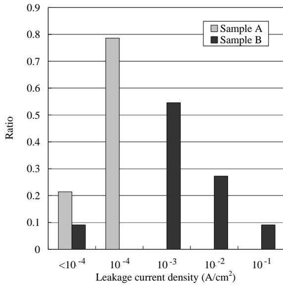
Fig. 3. Histogram of leakage current densities at -5V for Schottky contacts on the samples.
