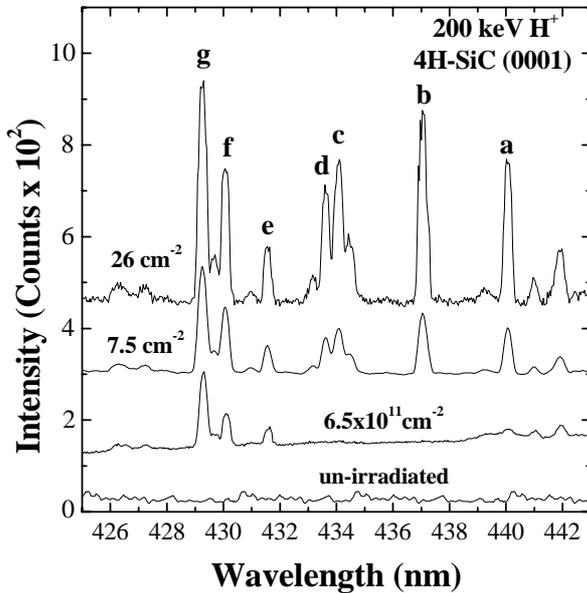
Fig.1: LTPL spectra (40 K) of the un-irradiated 4H-SiC sample and of different fluence irradiated
