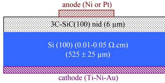
Fig. 1: Schematic view of the vertical diodes.
