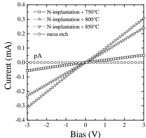
Fig. 2: I-V curves measured in structures isolated by mesa etch or nitrogen implantation. Thermal annealing leads to a decrease of the sheet resistance of the N-implanted region
