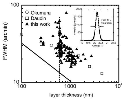
Fig. 1: Rocking curve linewidth of cubic GaN epilayers grown on 3C-SiC substrates versus thickness of the cubic epilayers.
