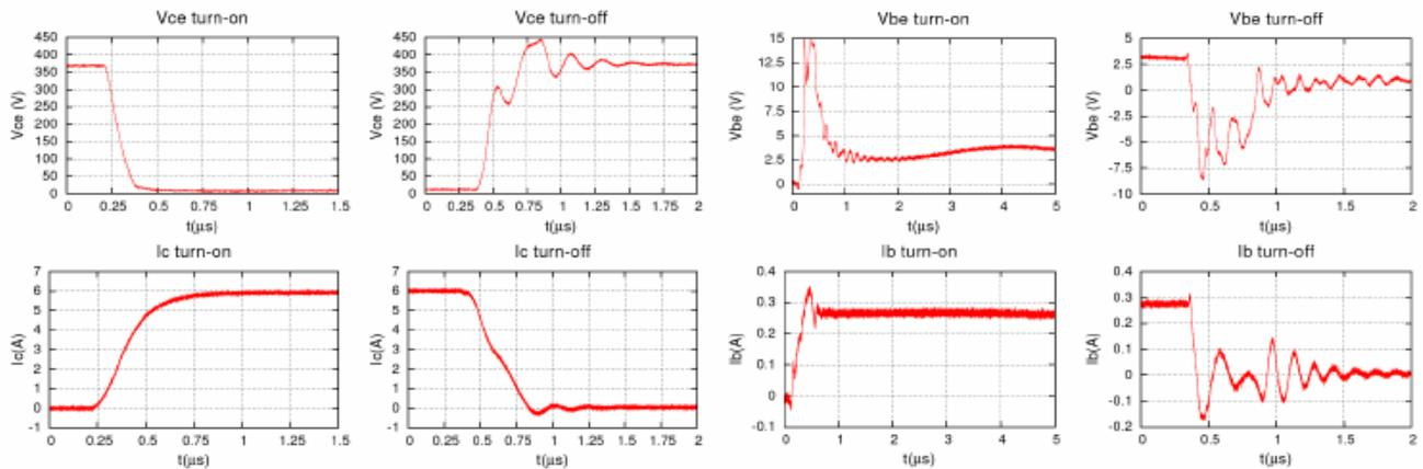
Fig 5: Switching waveform : collector (left), base (right) using discrete driver.
