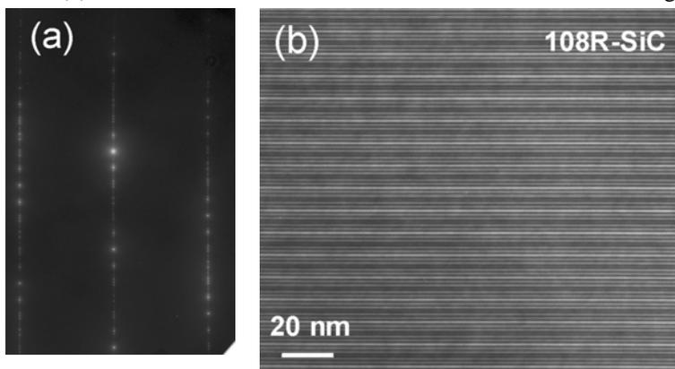
Fig. 4: (a) SADP revealing the formation of 108R-SiC (b) conventional XTEM image.
