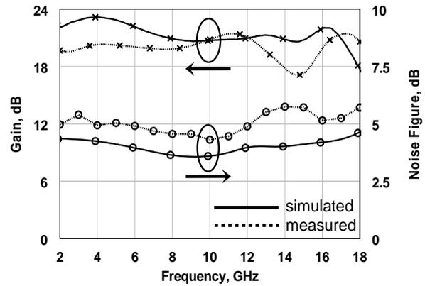
Fig. 3: Broadband LNA simulated and measured performance, small-signal gain and noise figure
