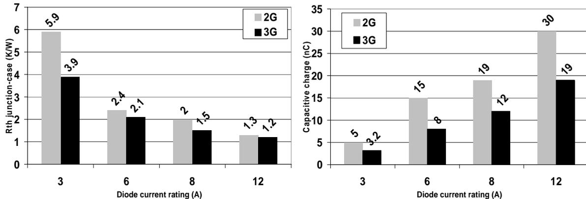
Fig. 1: Improvement of thermal resistance chip junction-to-case ( $R_{th,jc}$ , left) and device capacitances (right) for second and third generation SiC diodes. (Please note, that diodes with same current rating are compared, not with same active area!)
