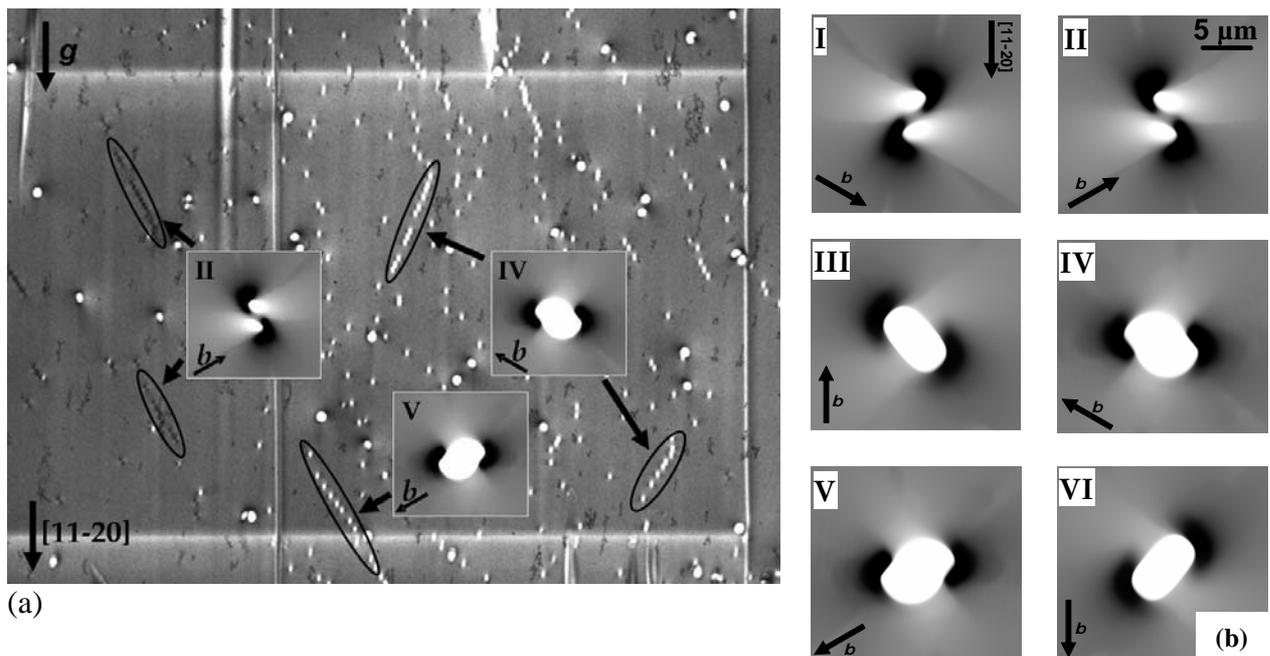
Fig. 2: (a) 11-2 12 Grazing incidence monochromatic image recorded from an epilayer grown on a 3 inch, 4H-SiC wafer showing TSDs and six different kinds of TEDs some of which aggregate into small angle boundaries; (b) simulations of the six types of TED.
