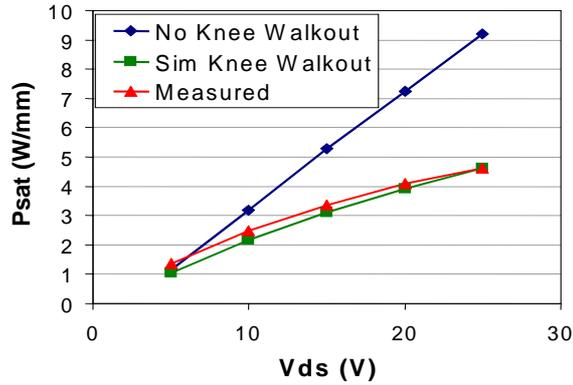
Fig.5: Experimental and simulated RF power vs drain supply voltage for GaN HFET (no field plate)
