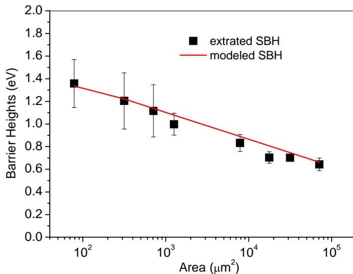
Fig. 3: Schottky Barrier Heights (SBH) versus area of the diodes. The continuous line is a fit to the model.
