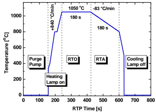
Fig.2: Schematics of the *in-situ* RTP sequence, including Rapid Thermal Oxidation (RTO) and Rapid Thermal Anneal (RTA) steps.
