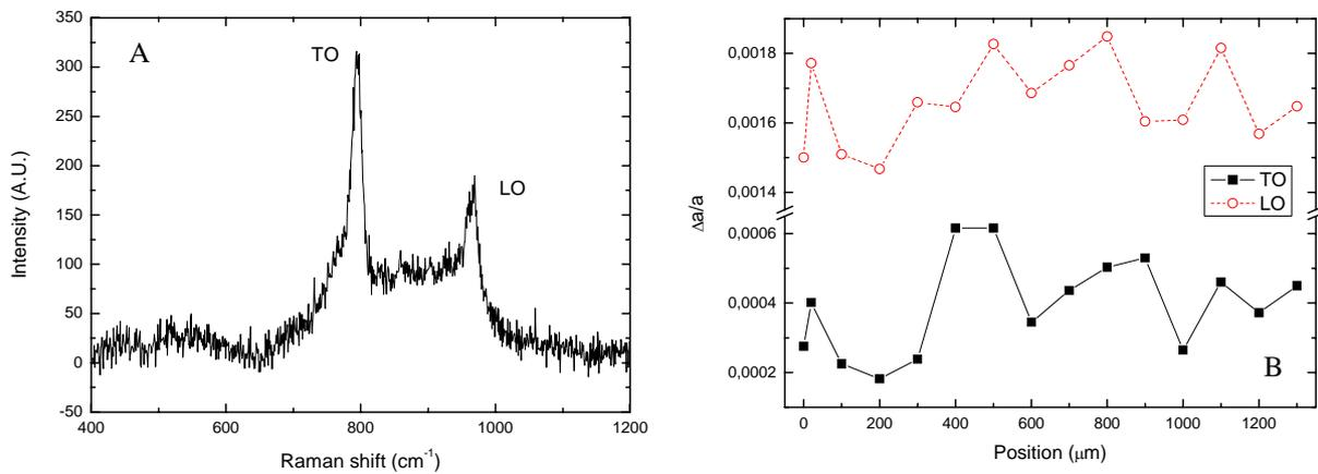
Fig.2: Typical Raman spectrum obtained on a freestaing membrane (A). Strain values obtained from Raman fittings in different point of the freestaing membrane (B)
