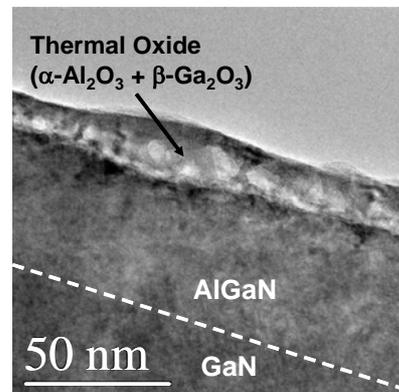
Fig. 4: Cross section TEM image of the AlGaN/GaN sample after annealing in  $\text{O}_2$  at 900°C
