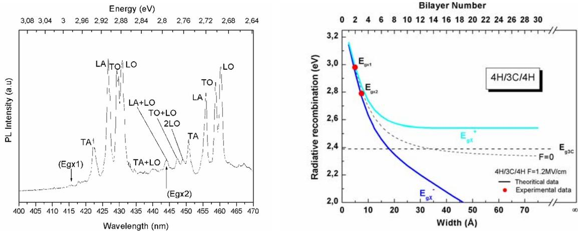
Fig. 1: Example of LPTL spectra collected at 5K, respectively on the 4H-SiC epitaxial layer considered in this work. From the phonon-assisted TA, LA, TO, LO replicas, two excitonic energy gaps indicative of 2 and 3 BLs thick 3C lamellae are deduced.
