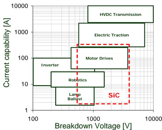
Fig. 1: Applications for Power Devices in Si and SiC.
