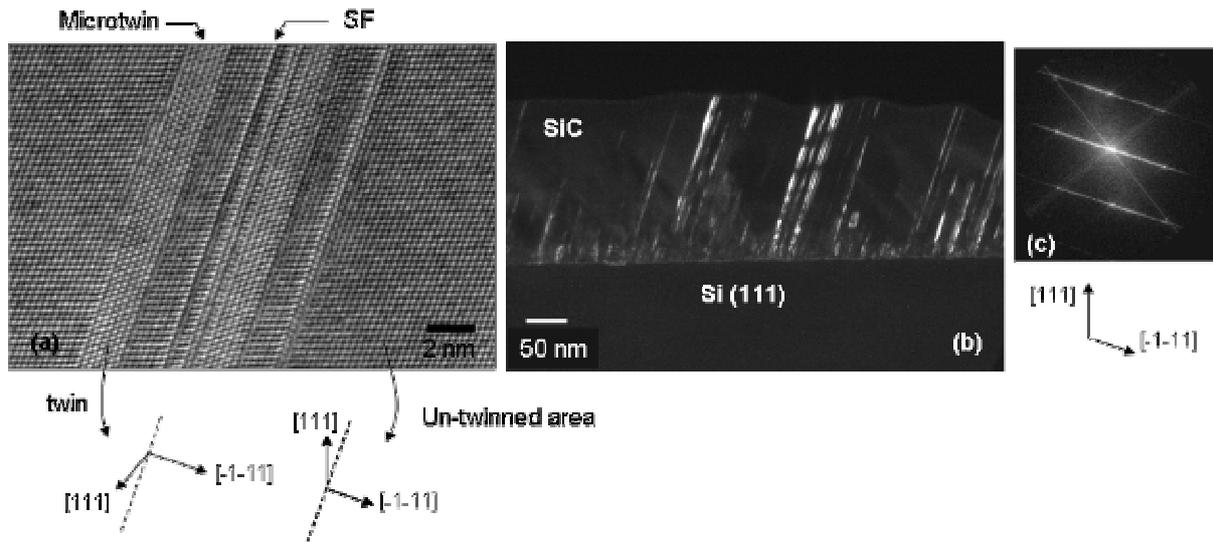
Fig.1: (a) High resolution micrograph of stacking faults and microtwins along (-1-11) planes. (b) Dark field imaging of the planar defects. (c) Diffraction pattern along the [1-10] zone axis with diffraction lines due to SFs.
