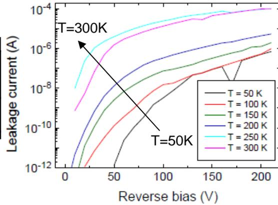
Fig. 2: Changes in leakage current as a function of the reverse bias voltage at various operating temperatures.
