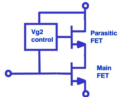
Fig. 4: Schematic diagram of virtual gate model of GaN HFET.
