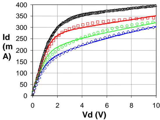
Fig.3: Measured  $I_d$ - $V_{ds}$  characteristics for an AlGaIn/GaN FET in pulsed operation, for various quiescent biases. The top curve corresponds to dc operation. Also shown are simulated curves from a physics-based model.
