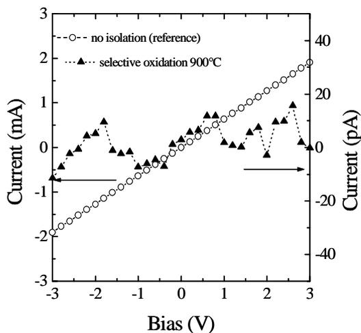
Fig. 3: I-V curves measured in structures isolated by selective oxidation at 900°C. The I-V curve of the reference sample (no isolation) is also reported
