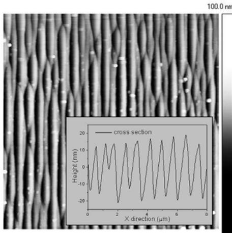
Fig. 1: AFM image of step bunching structures and the corresponding height across the ripples.
