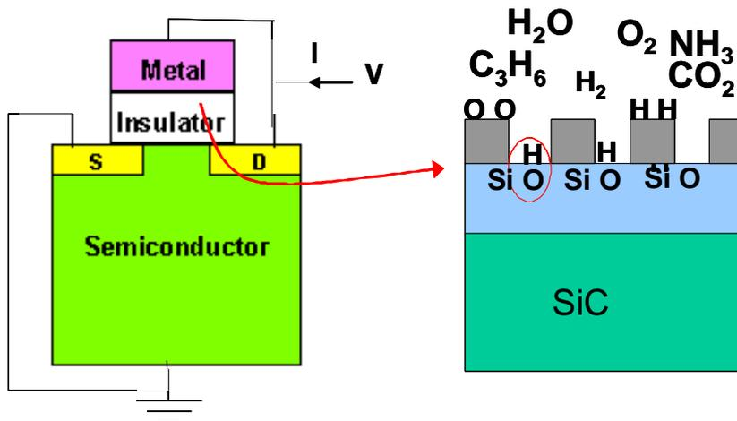
Fig. 1: Schematic picture of a field effect transistor as a sensor device and a close up of the gate area (to the right). Charging of the gate area by gas molecules create an electric field which changes the current through the transistor.
