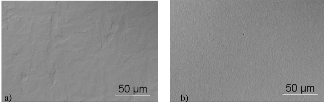
Fig. 1: Optical microscope image of a 3C-SiC surface grown on Si(001) substrate on-axis (a) and on Si(001) substrate 4° off-axis towards [001] direction (b).
