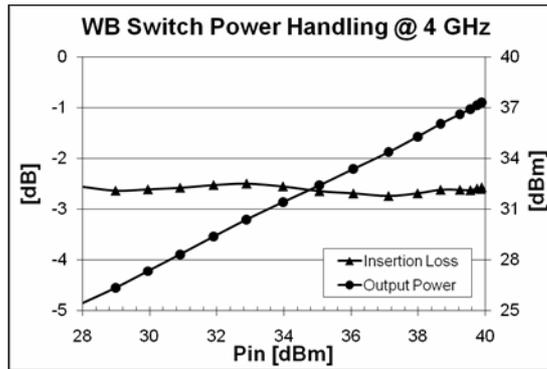
Fig. 7: Broadband Switch measured performance: output power and insertion loss
