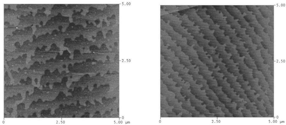
Fig. 2: AFM image from 3C-SiC layers grown on substrate Type I (a) and IV (b), respectively, showing different terrace width.
