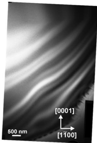
Fig. 3: A TEM micrographs from the layer grown on C face 6H-SiC substrate using pure Si as a solvent.
