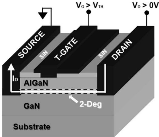
Fig. 1: Schematic structure of studied HEMTs. It is possible to note the field plate over the Gate contact (T-shape Gate). Artwork not in scale.
