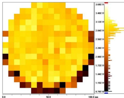
Fig. 4: Corema resistivity map of SI 100 mm wafer with a resistivity of  $2.9 \text{E}11 \text{ } \Omega\text{-cm}$ .
