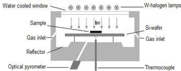
Fig.1: Schematics of the AsOne RTP furnace used in this work.
