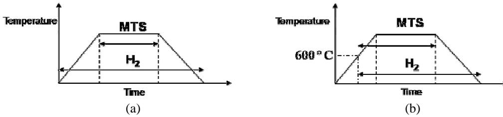
Fig. 1. Two different precursor feeding procedures: (a) procedure I, (b) procedure II.
