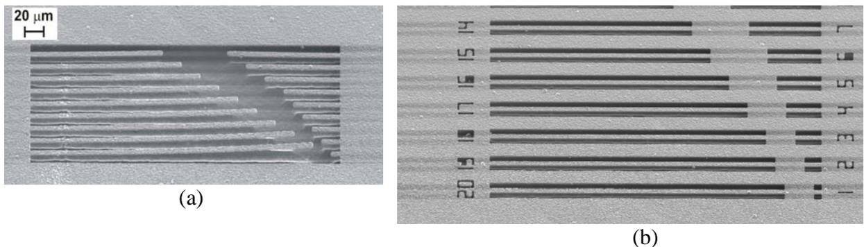
Fig.3: SEM micrographs of (a) cantilevers and (b) bridges from poly 3C-SiC 1.5  $\mu\text{m}$  thick films
