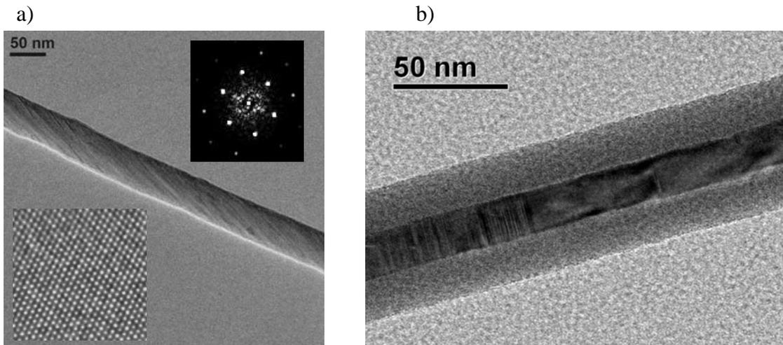
Fig. 2: TEM images of a typical  $\beta$ -SiC NW (a) and a typical  $\beta$ -SiC / SiO<sub>2</sub> core/shell NW (b). A high resolution image of a perfect region and the corresponding diffractogram are shown as inset in (a).
