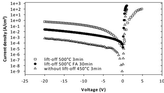
Fig. 3: Best J/V characteristics for SBD made by lift-off or using standard photolithography process at various temperature.
