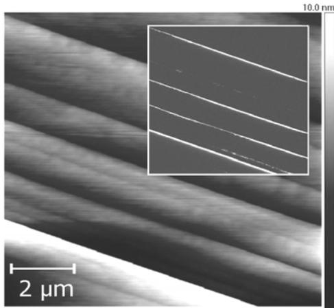
Fig. 1: Morphology taken by C-AFM. Insert shows corresponding current map in the same scan area, where bright lines measure leakage current in excess of 1 pA.
