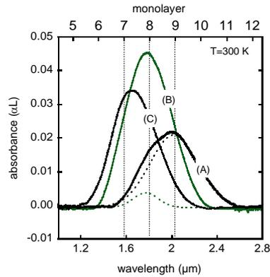
Fig. 2: Optical absorption spectra of the intersubband transitions in cubic GaN/AlN short period multiple quantum wells (MQWs).
