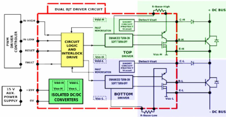
Fig 4: Fabricated discrete BJT driver topology (dashed rectangle to be integrated using SOI technology).
