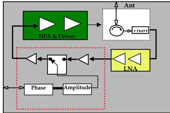
Fig. 1: Typical T/R module schematic (separate architecture)
