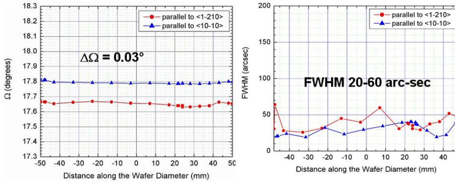
Fig. 3: X-ray evaluation of 100 mm 6H-SiC wafer Lattice Curvature ( $\Delta\Omega$ ) =  $0.03^\circ$ . FWHM = 20-60 arc-second in 100 mm area.
