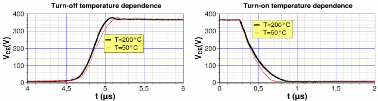
Fig. 6: Turn-off (left) and turn-on (right) dependence on temperature (50°C and 200°C).
