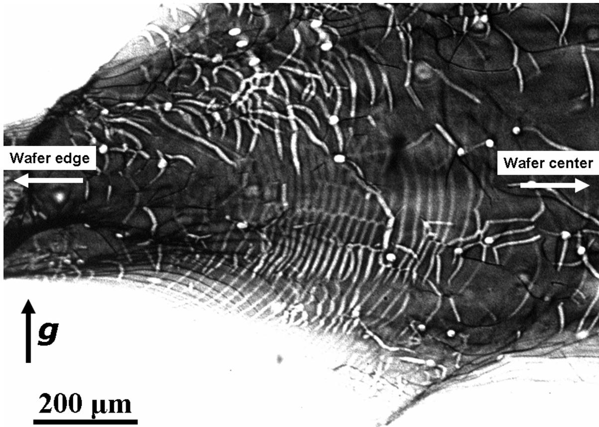
Fig. 4: Monochromatic topograph recorded from a 4H-SiC substrate. Note the concentric loops of white contrast BPDs which indicate that they are all of the same sign and that they are formed via deformation processes that occur near the wafer edge and propagate towards the wafer interior.
