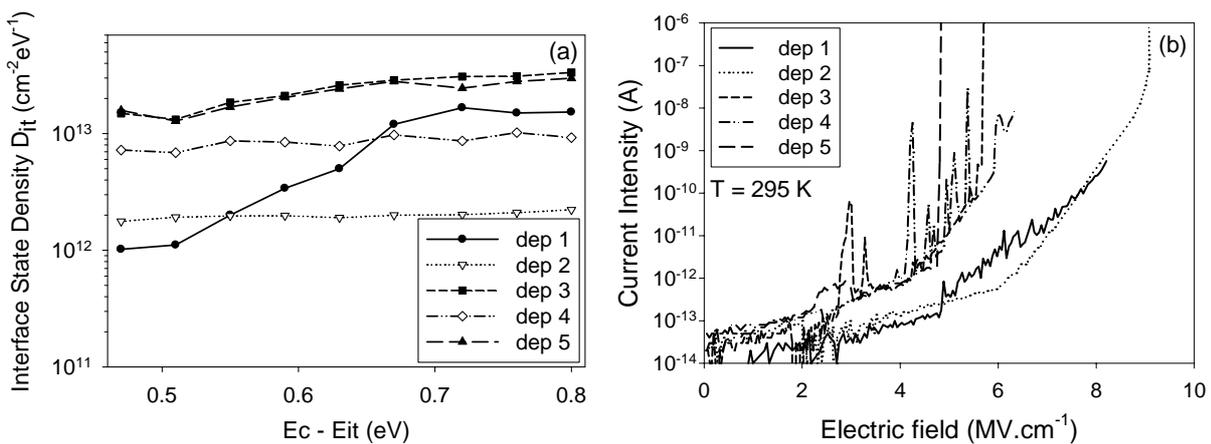
Fig. 2. Interface state density  $D_{it}$  as a function of the energy position (a) and I-V characteristics (b) of 3C-SiC MOS capacitors fabricated by PECVD and post oxidized in N<sub>2</sub>O (1100°C), wet, and dry oxygen (950°C) for 3 hours (dep 1-3) or post annealed in N<sub>2</sub> at 950°C and 1100°C for 3 hours (dep 4 and 5).
