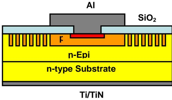
Fig. 1: Cross-sectional structure of a pn diode: An Al implanted 1μm-depth box profile with  $1 \times 10^{18}/\text{cm}^3$  is fabricated in n-type epitaxial layer with  $[N]=7 \times 10^{15}/\text{cm}^3$ . The diode is surrounded by six guard rings with 1μm-width. Al electrode is contacted to 0.2μm-thick  $p^+$  layer with  $[Al] = 1 \times 10^{20}/\text{cm}^3$ .
