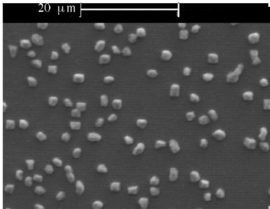
Fig.2: SEM image of SiC grown at 1200°, showing hillocks
