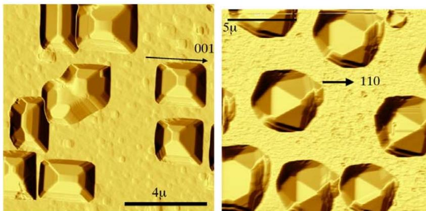
Fig.3: AFM images of SiC surface grown at 1200 on Si 001 (left) and Si (111) right
