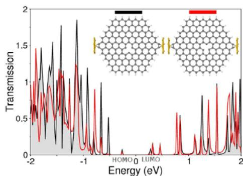
Fig. 2: Transmission as a function of energy by means of the Extended Hückel method for two equivalent contact configurations that differ only in the position with respect to the defected site.
