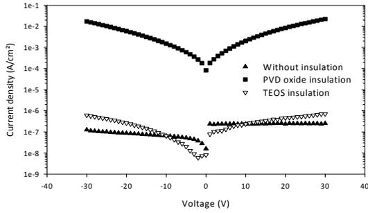
Fig. 1: Comparison of J(V) on "Schottky to Schottky" structures with or without an insulation step. (Furnace annealed at 400°C during 30min).
