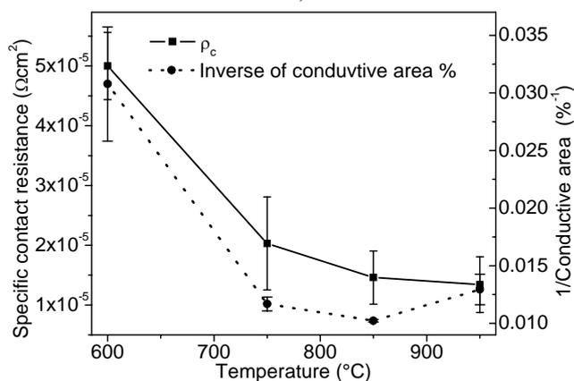
Fig. 1: Specific contact resistance (solid curve), and inverse of the effective contact area (dotted curve) vs. temperature. Measured on Ni-based Ohmic contacts on 3C-SiC grown by VLS.
