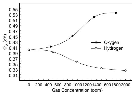
Fig. 4: Variation in barrier height with hydrogen and oxygen exposure.
