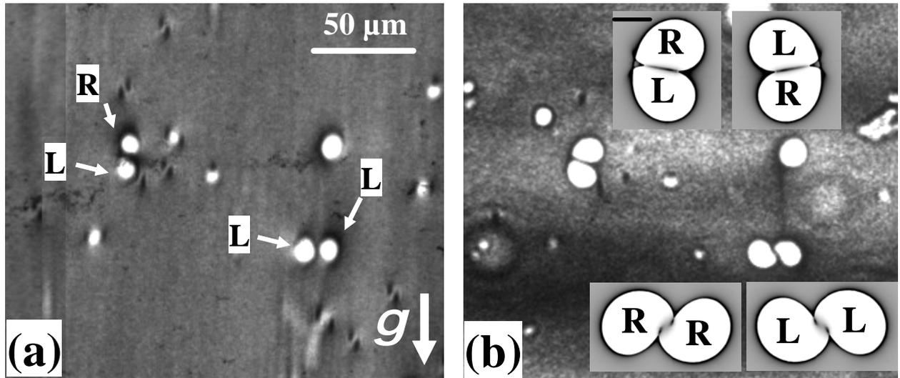
Fig. 1: X-ray topographs recorded using monochromatic synchrotron radiation from a 4H-SiC substrate. (a) recorded in grazing incidence; (b) recorded in back reflection (insets show simulations). Detailed ray tracing simulations enable determination of both the magnitude and sign of the TSDs. L indicates left-handed, R right-handed.
