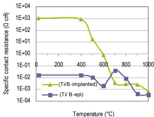
Fig. 2: Specific contact resistances of Ti contacts to boron-implanted and epitaxial boron-doped diamond as a function of PDA temperature.
