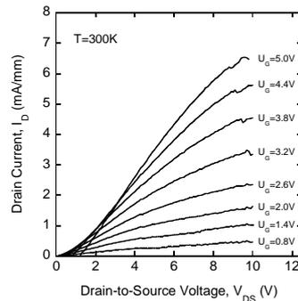
Fig. 3:  $I_{DS}$ - $V_{DS}$  characteristics of a cubic AlGaN/GaN HFET measured at room temperature after subtraction of the c-GaN buffer conductivity.
