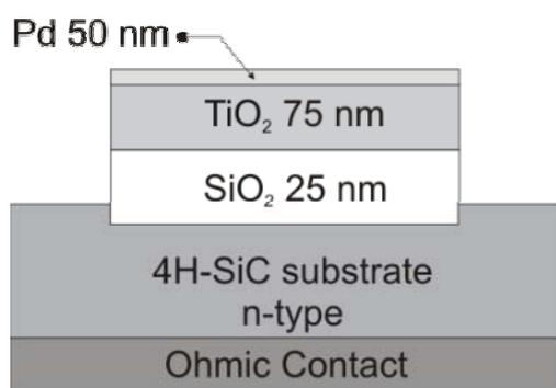
Fig. 1: Schematic cross section of a capacitive gas sensor.
