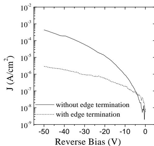
Fig. 2: Reverse characteristics of Ni/Au Schottky diodes with and without non-annealed Mg-implanted guard ring.
