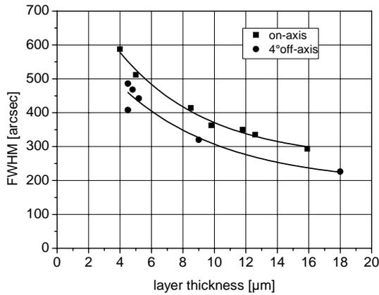
Fig. 2: FWHM of the rocking curve in dependence on the epitaxial layer thickness and substrate orientation
