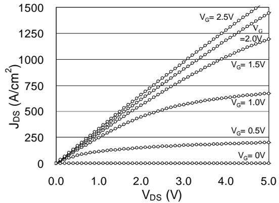
Fig. 4: Simulated output characteristic of DGTJFET with anisotropic conditions for a Si-face SiC wafer.
