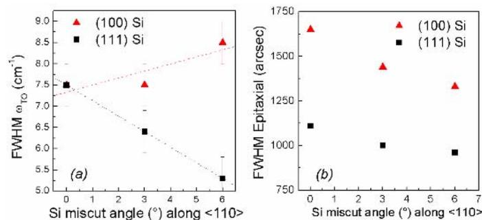
Fig. 3: FWHM trends of Raman TO 3C-SiC phonon mode and of epitaxial 3C-SiC XRD peak. Sample thickness is about 3  $\mu\text{m}$ .
