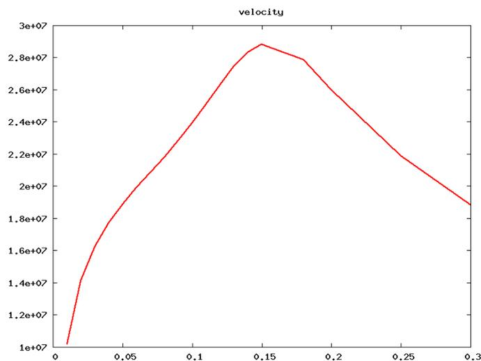
Fig. 2: Calculated electron velocity (cm/s) as function of the applied electric field (MV/cm) in bulk wurtzite GaN at 300 K.
