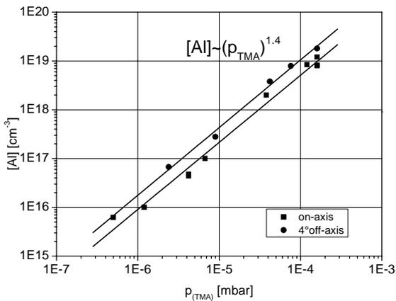
Fig. 4: Aluminum concentration (SIMS) in dependence on the Trimethylaluminium –partial pressure in 3C-SiC layers on Si(001) on-axis and 4° off-axis
