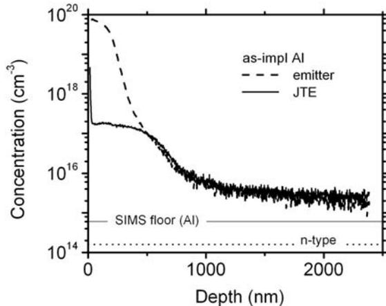
Fig. 1. SIMS profiles of as-implanted Al in emitter and JTE areas. Measurement floor and n-type concentration in the epitaxial 4H-SiC are also shown for comparison.
