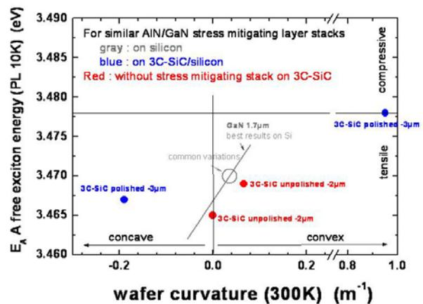
Fig.4: Comparison of the residual strain measured by PL obtained on GaN films grown on 3C-SiC(111) epilayers
