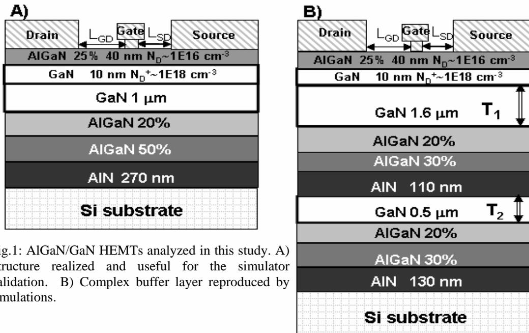
Fig.1: AlGaIn/GaN HEMTs analyzed in this study. A) Structure realized and useful for the simulator validation. B) Complex buffer layer reproduced by simulations.
