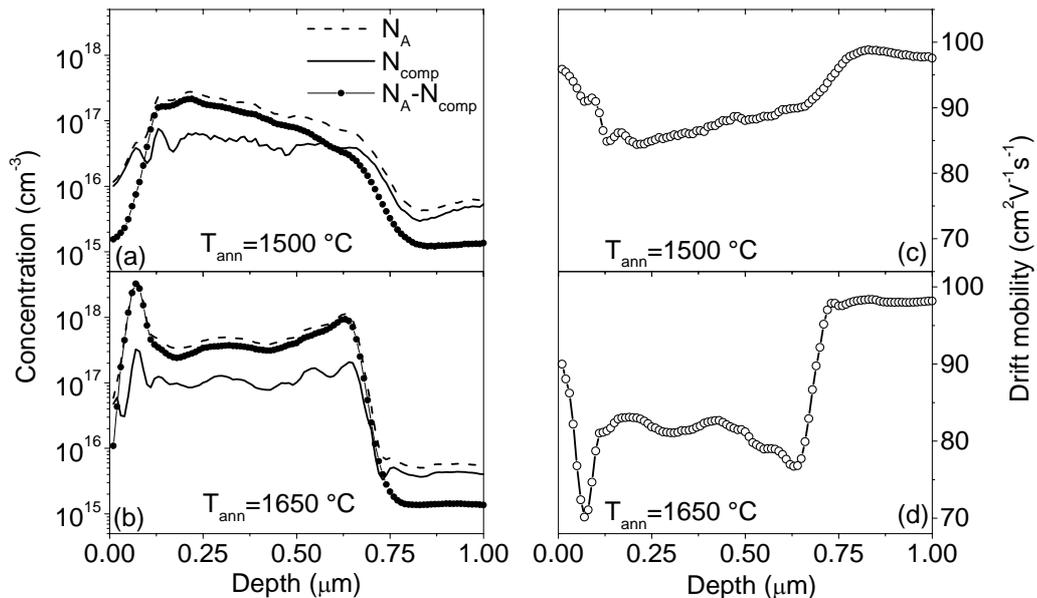
Fig. 1: Measured profiles of  $N_A$ ,  $N_{comp}$  and of the net dopant concentration ( $N_A - N_{comp}$ ) on Al implanted 4H-SiC after annealing at 1500 °C (a) and 1650 °C (b). The evaluated drift mobility profiles for the two annealing temperatures are reported in (c) and (d), respectively.
