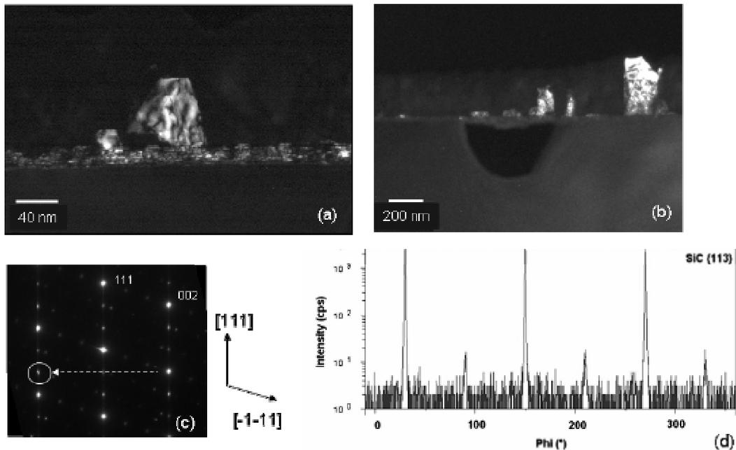
Fig.2: (a) Dark field imaging of a small basal twin (65 nm width) in a sample elaborated with high propane flow rate during carbonization. (b) Dark field imaging of large basal twins (300 nm width) in a sample elaborated with low propane flow rate. (c) Diffraction pattern with projected spots due to the basal twinning. (d) Azimuthal XRD scan recorded along the asymmetric {113} direction on the sample with low propane flow rate.
