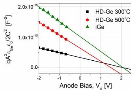
Fig 4: C-V characteristics of the MBE Ge/SiC layers
