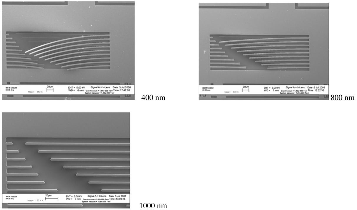
Fig.1: Cantilevers obtained in different zones of the same SiC film with different thickness
