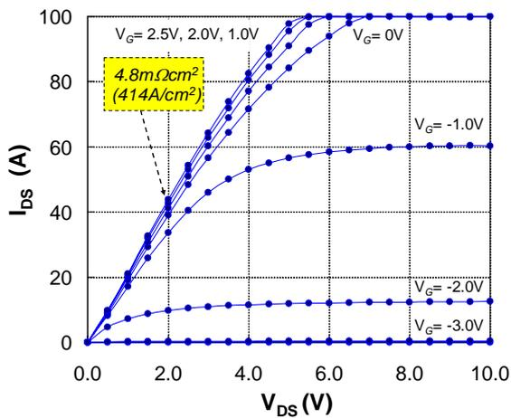
Fig. 7: Output characteristic of fabricated 9.5  $\mu\text{m}$  cell pitch normally-on 4H-SiC DGTJFET.
