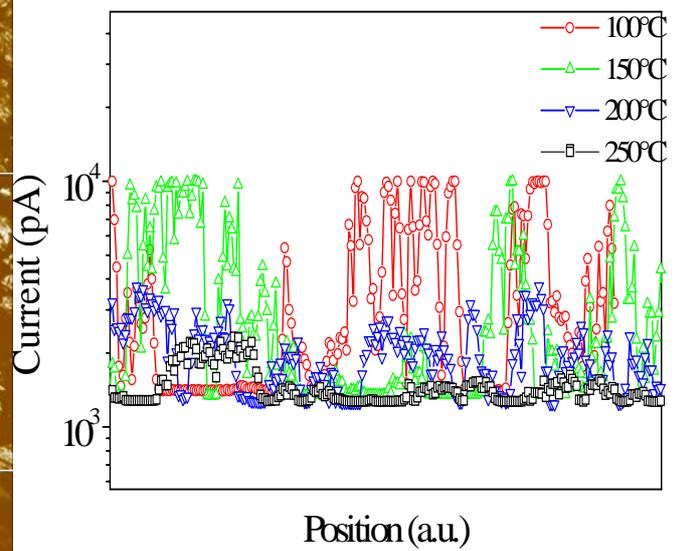
Fig.: 3: Current profiles across the grain and grain boundaries at different temperatures
