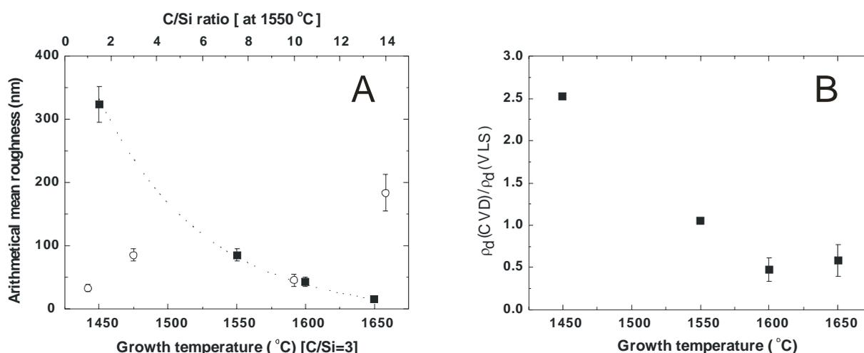
Fig. 2: Arithmetical mean roughness of the surfaces of CVD homoepitaxial layers (a) versus the applied growth temperature (■) and the C/Si ratio (○). The  $\rho_D(\text{CVD})/\rho_D(\text{VLS})$  defect density fraction dependence on the growth temperature is shown in figure b). The error bars correspond to statistical errors. The dashed line is guide for the eyes in figure a).
