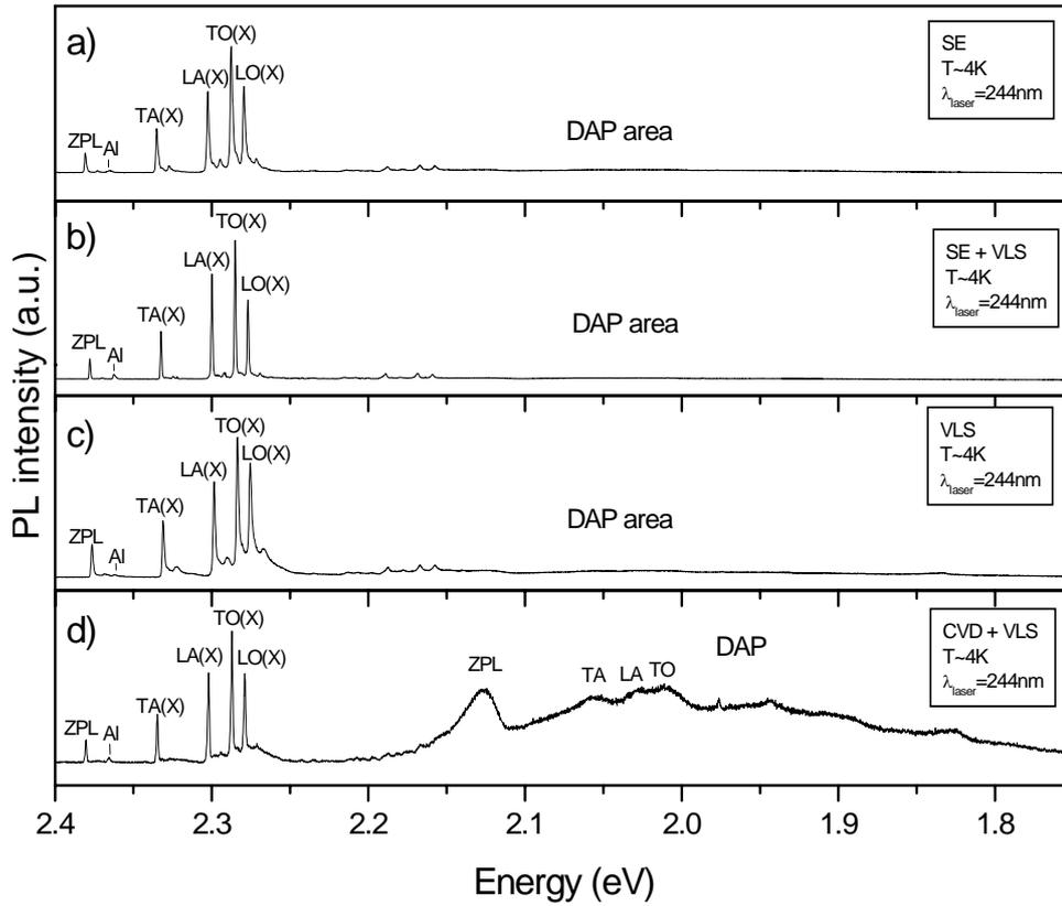
Fig. 1: LTPL spectra collected for different 3C-SiC samples grown using a) SE, b) SE on a VLS seed, c) an optimised VLS technique and d) CVD re-growth on a VLS seed.
