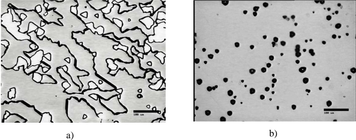
Fig.1: Optical microscope image in transmission mode taken from samples grown on substrate Type I (a) and IV (b), respectively. The scale bar is 100  $\mu\text{m}$ . The colors on the picture are not original because of the grey scale, the grey correspond to 3C-SiC and white to 6H-SiC inclusion.
