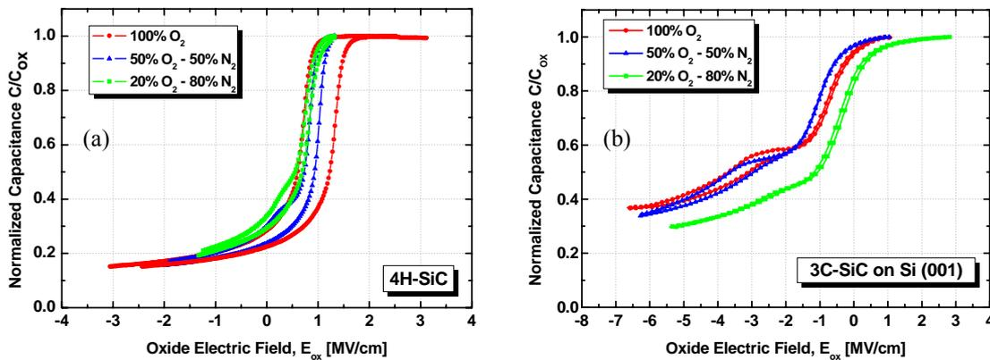
Fig.3: Comparison of the high frequency ( $\omega = 1$  MHz) C-V characteristics collected for oxides grown on 4H-SiC (a) and 3C-SiC (b) by rapid thermal oxidation during 180 s for different O<sub>2</sub>/N<sub>2</sub> mixtures (1050 °C) and annealed in N<sub>2</sub> for 180 s.
