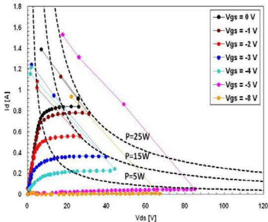
Fig. 5: I-V Output curves in 100 ns TLP regime to evaluate the breakdown points at different  $V_{GS}$ . ( $W = 1000\mu\text{m}$ ,  $L_G = 0.5\mu\text{m}$ , SiC).
