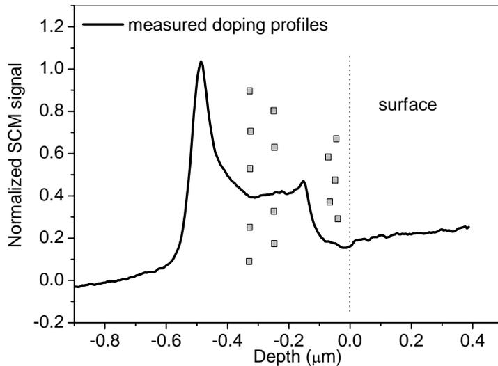
Fig. 3: Measured SCM signals, filled squares illustrate the precipitates which were found in the TEM image.
