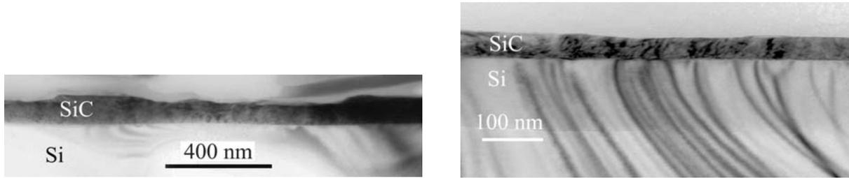
Fig. 1: TEM images of SiC sample grown at 1200°C (left) and 1250 °C (right)
