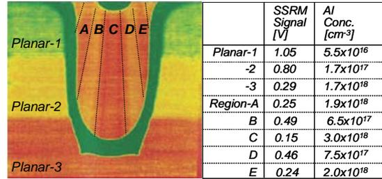
Fig. 2: 2D Al-dopant distributions in the embedded trench structure (SIMS and SSRM investigations).
