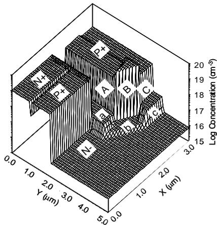
Fig. 3: N and Al dopant concentration 3D profiles of embedded trench structure on C-face SiC wafer.
