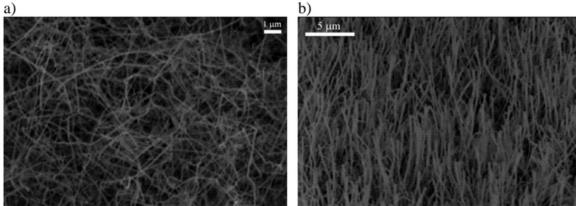
Fig. 1: SEM image of 3C-SiC wires, a) pure nanowires, b) core-shell nanowires
