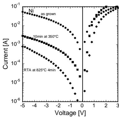
Fig. 3: Room temperature current voltage (I-V) characteristics of a Ni-Schottky contact on cubic GaN before annealing (full circles), after annealing in air at 350°C (full squares and after RTA at 25°C (full diamonds).
