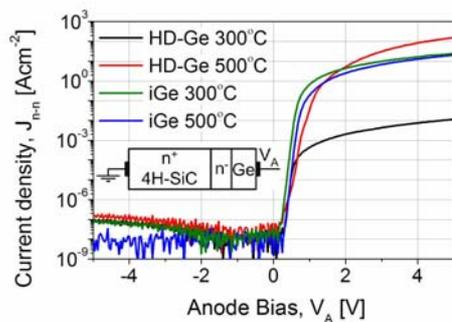
Fig 3: Semi-log I-V characteristics of the MBE Ge/SiC layers
