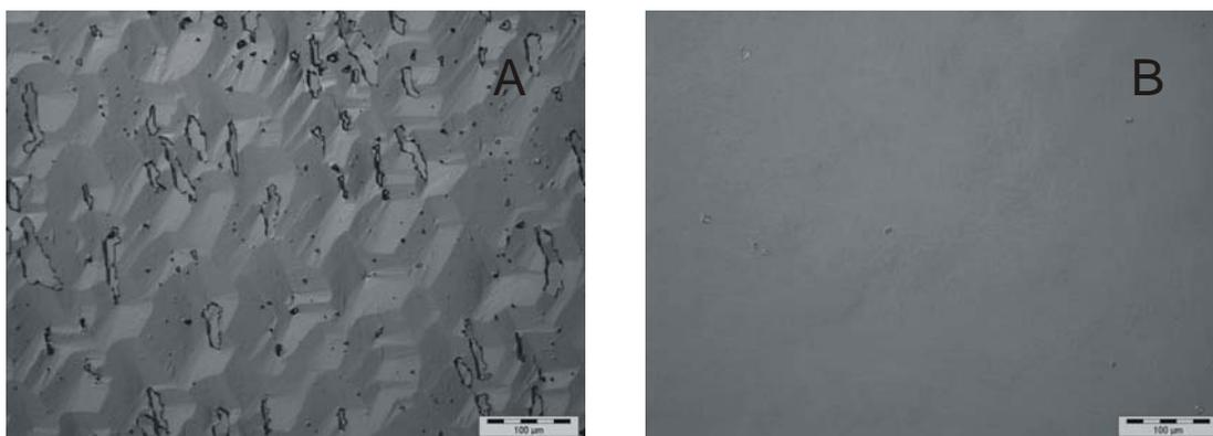
Fig. 1: The surface morphology of CVD homoepitaxial layers grown on VLS seeds by applying a)  $T=1550\text{ °C}$  and b)  $T=1650\text{ °C}$  growth temperature with C/Si ratio of 3.
