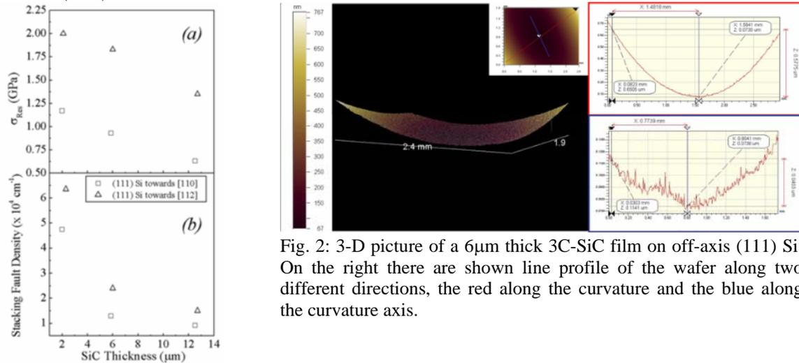
Fig. 1: (a) Average residual stress and (b) stacking fault density of 3C-SiC films grown on (111) Si with off-cut axis towards [110] and towards [112].
