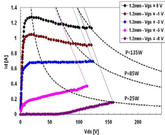
Fig. 6: I-V Output curves of SiC HEMT ( $W = 1200\mu\text{m}$ ) under 100 ns TLP regime.  $V_{GS}$  values are reported in the label.
