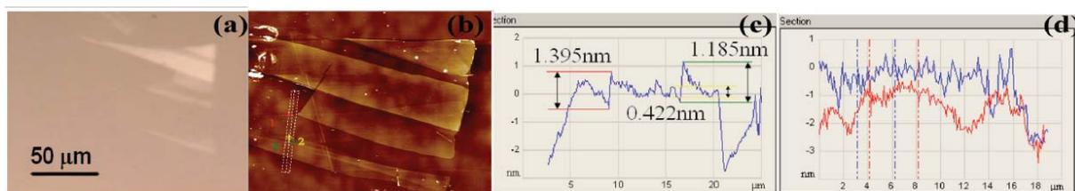
Fig.1: Graphene deposited on SiC showing optical micrograph in (a), tapping mode AFM micrograph in (b), an AFM linescan showing the relative thickness of deposited flakes in (c) and a linescan in (d) shows that graphene follows the surface morphology of SiC, the blue linescan is taken on graphene on SiC while the red linescan is taken on bare SiC substrate.
