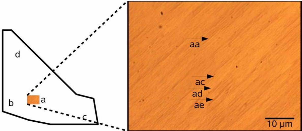
Fig.1 Schematics of the FLG sample investigated in this work, with expanded microscope view.
