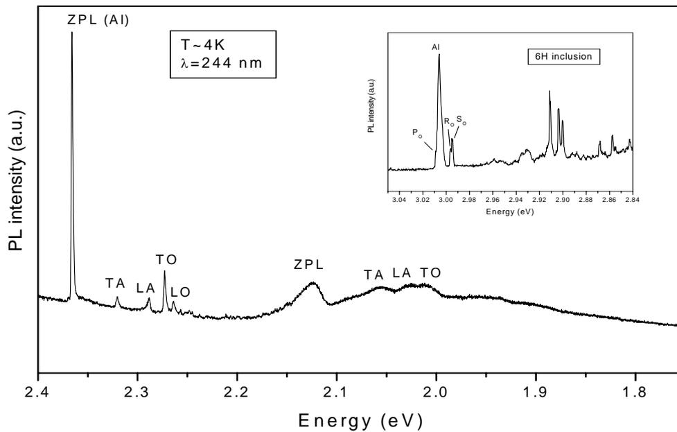
Fig. 2: LTPL spectra collected for an Al-doped sample grown using SE. The first peak corresponds to Al bound excitons. The other ones are one phonon replicas. The insert shows a 6H-SiC inclusion with again a high level of Al concentration.
