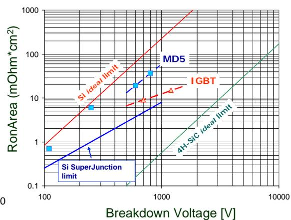
Fig. 2: From Si to SiC. Trade-off curves of  $R_{on}$  vs  $V_B$  for power devices
