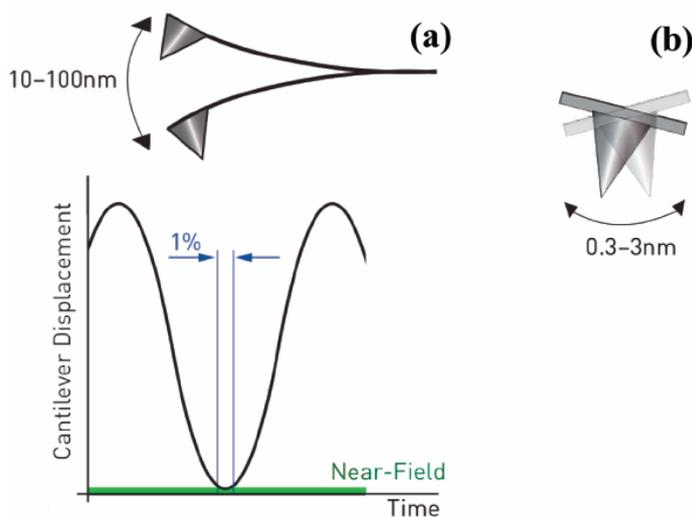
Fig. 3: A schematic comparing tip movements in (a) Tapping mode and (b) in Torsional resonance mode. The tip is in close proximity to the sample for approximately 1% of the oscillation cycle when using standard Tapping mode. In comparison the tip can be in close proximity to the surface all of the time when using Torsional resonance mode with small oscillation amplitude.
