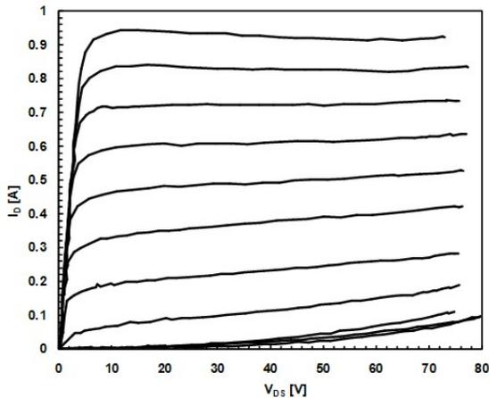
Fig. 3: I-V curves in 100 ns-TLP regime. Device width  $W = 1\text{ mm}$ , SiCopSiC. Gate bias:  $0\text{ V} \leq V_{GS} \leq -5\text{ V}$ , step 0.5 V.
