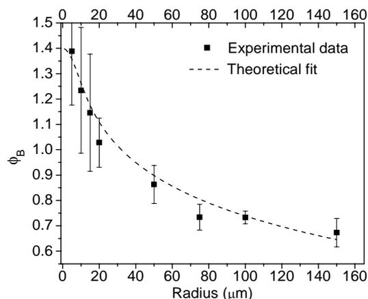
Fig. 2: SBH vs. contact radius, measured on a Au/3C/4H-SiC/ $\text{Ni}_2\text{Si}$  structure. The dashed curve is a fit to a model that relates the SBH to the defect density.
