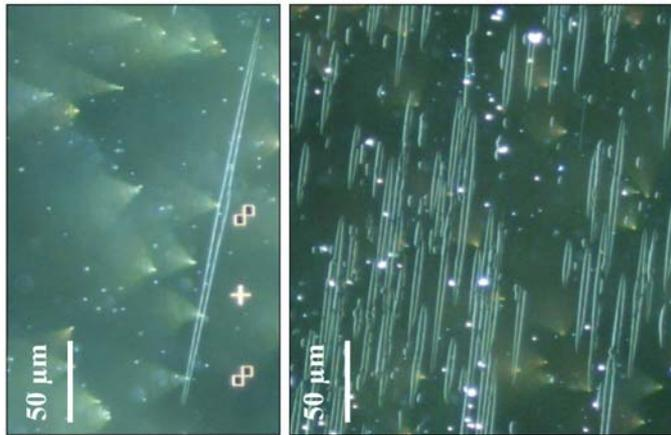
Fig. 1: Wide range Optical Microscopy view of samples covered by very long graphene ribbons from 30 to 300  $\mu\text{m}$  long and 5  $\mu\text{m}$  large depending on the sublimation time. Higher density of ribbons is encountered where higher density of defects on the surface of the SiC substrate.
