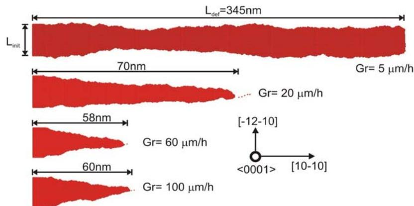
Fig.1: Plan view of the grown (1,-1,+1,-1) defects for different growth rate. We note that, at the slowest growth rate of  $Gr=5 \mu\text{m/h}$  the defect never closes, i.e. the defect length  $L_{def}$  exceeds the computational box. The initial extension of the defect along the  $[-12-10]$  direction ( $L_{init}$ ) is the same for all the simulations. It is the equivalent of the panchromatic cathodoluminescence experimental images ( see, for example Fig.1 of [11])
