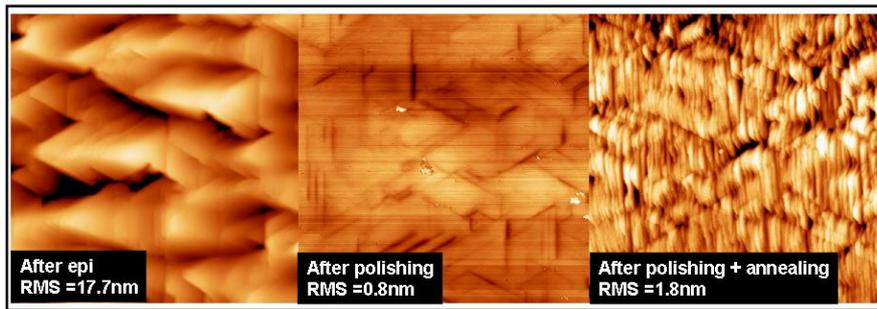
Fig.2: Evolution of the surface morphology of 3C-SiC epilayer grown on 2'' 4°off silicon substrate.
