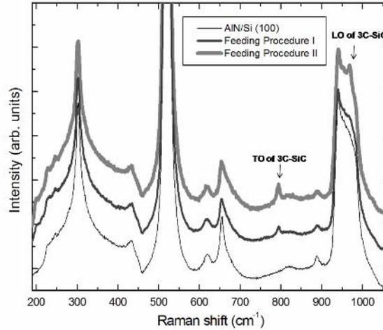
Fig. 2. Raman spectra of an AlN/Si (100) substrate, and of a series of SiC films on AlN/Si (100) obtained by different feeding procedures deposited at 1200 °C and H<sub>2</sub>/MTS flow rate ratio at 100.
