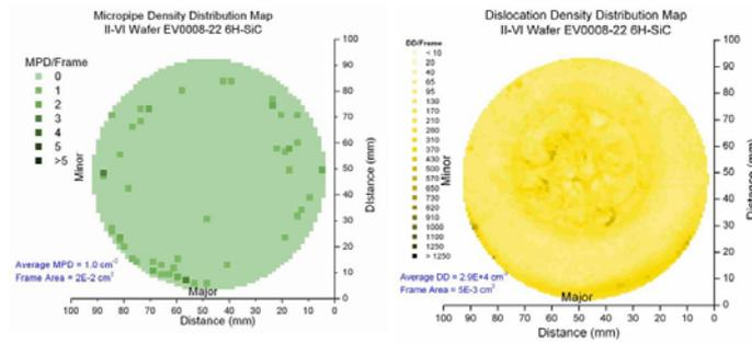
Fig. 2: - Left - Micropipe density map (MPD) of a 100 mm wafer. MPD =  $1.0 \text{ cm}^{-2}$  Right – Dislocation density (DD) map of 100 mm wafer. DD =  $2.9 \text{E}4 \text{ cm}^{-2}$ .
