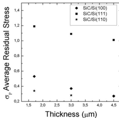
Fig. 4: Radius of curvature stress measurement as a function of thickness performed on 3C-SiC film grown on different Si substrate.
