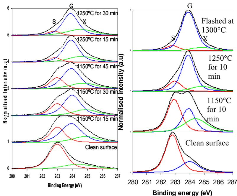
Fig. 1. Stacked, curve fitted plot of XPS data for the C1s peak, showing graphene growth during (a) direct current annealing from 1150°C to 1250°C, and (b) e-beam annealing from 1150°C to 1300°C
