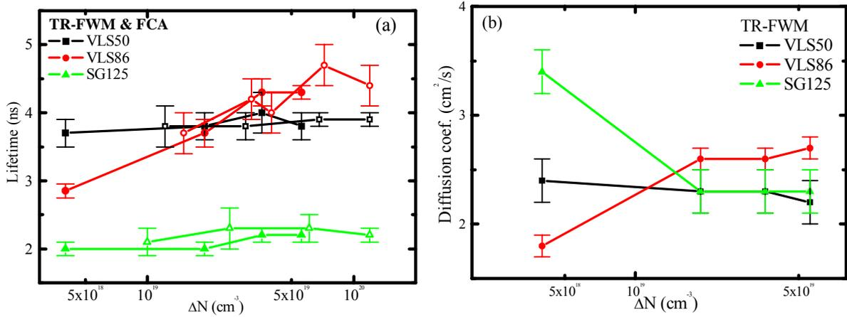
Fig. 1: Carrier lifetime  $\tau_R$  (a) and ambipolar diffusion coefficient  $D_a$  (b) as a function of excess carrier density  $\Delta N$  at room temperature.
