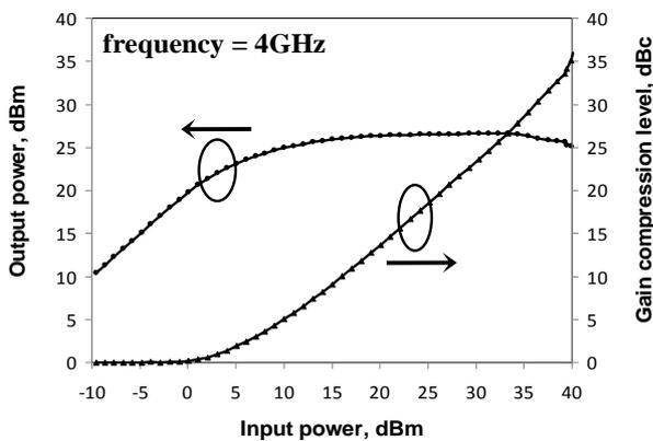
Fig. 4: Broadband LNA measured performance, output power and compression
