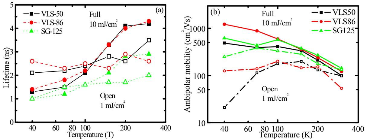
Fig. 2 Temperature dependencies of carrier lifetime (a) and ambipolar mobility (b) at low (1  $\text{mJ}/\text{cm}^2$ , open symbols) and high (10  $\text{mJ}/\text{cm}^2$ , full symbols) excitations.
