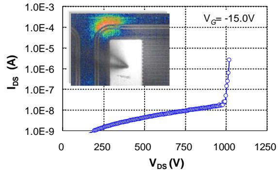
Fig. 6: Breakdown characteristics of normally-on 4H-SiC DGTJFET. Inset emission microscope image shows the breakdown location at the device termination edge.
