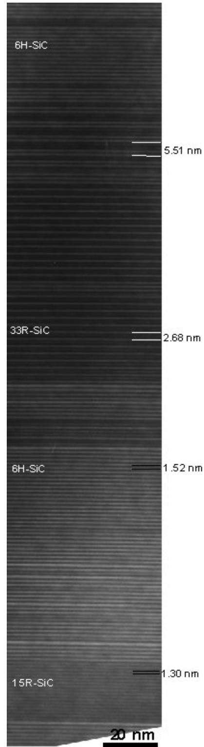
Fig 2: TEM micrograph of the layer grown on Si face substrate using a mixture of Si and Al as a solvent.
