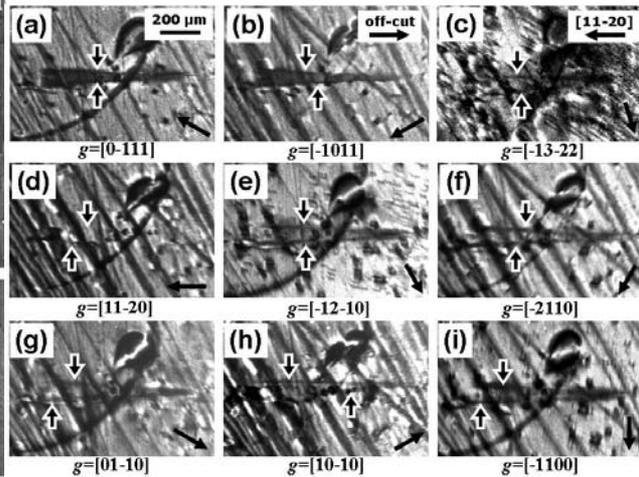
Fig. 6: Series of transmission topographs confirming the nature of the Frank partials and faults. The partial dislocations are out of contrast when  $\mathbf{g} \cdot \mathbf{b} = 0$  and  $\mathbf{g} \cdot \mathbf{b} \times \mathbf{l} = 0$ , where  $\mathbf{g}$  is the reflection vector,  $\mathbf{b}$  is the Burgers vector and  $\mathbf{l}$  is the line direction. The stacking fault is out of contrast when  $\mathbf{g} \cdot \mathbf{R} = 0$ , where  $\mathbf{R}$  is the fault vector.
