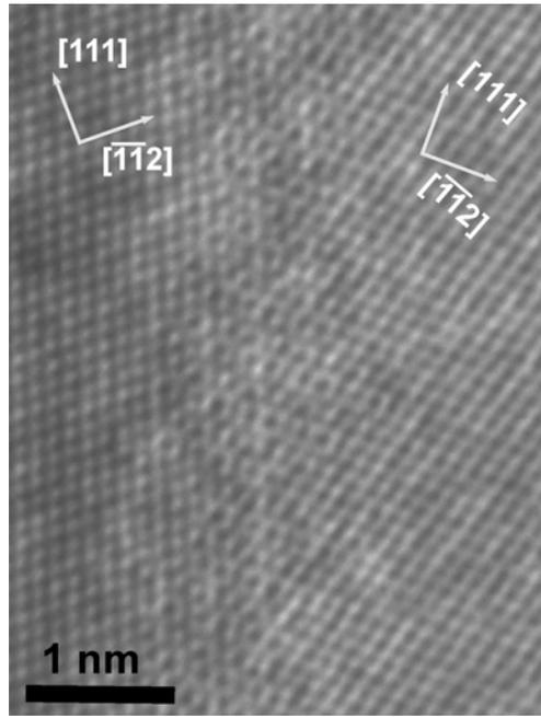
Fig. 2. HRTEM image of T<sub>2</sub>/T<sub>3</sub> DPB.
