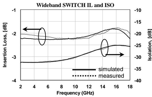
Fig. 6: Broadband Switch simulated and measured performance: insertion loss and isolation
