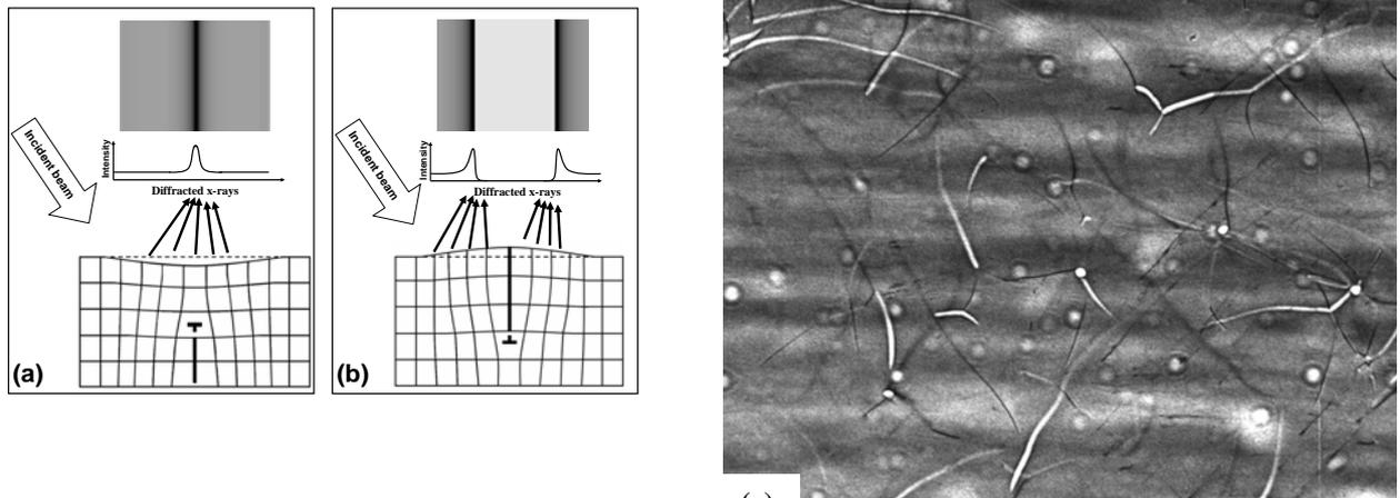
Fig. 3: (a) and (b) Schematics of back reflection ray tracing. (c) Simulations of BPDs in 4H-SiC. Simulation enables determination of both the sign and magnitude of the Burgers vector of the BPDs plane dislocations which appear as narrow dark lines or broad white lines with dark borders on the back reflection image (c).
