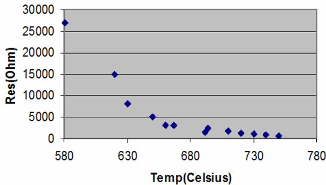
Fig. 2: 3C-SiC as a thermistor material. Measurements in the oven for temperature over 580°C.
