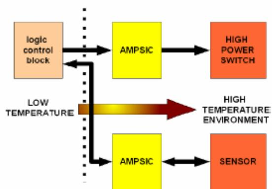
Fig 2: Proposed high temperature converters topology
