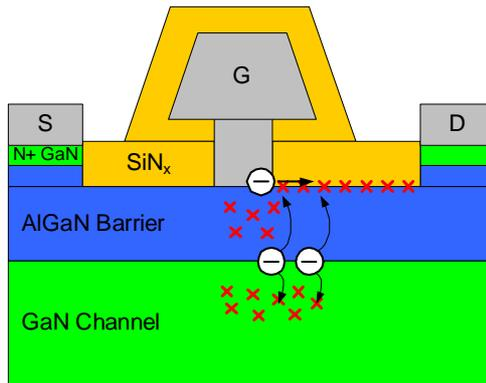
Fig.7: Illustration of various mechanisms for producing voltage-dependent charges adjacent to GaN HFET channel.
