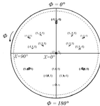
Fig. 2: X-Ray pole figure of 3C-SiC on Si(111) oriented
