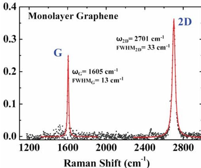
Fig. 2: Typical Raman spectrum of a monolayer graphene ribbon after subtraction of the SiC signal.
