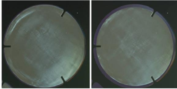
Fig. 1: Cross Polarizer images of two 100 mm wafers. Left – mottled contrast due to minor sub-grain. Right – no visible defect.
