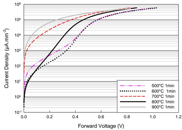
Fig. 2: J(V) forward characteristics represented for 0.17 mm<sup>2</sup> nickel anodes annealed between 500 °C and 900 °C.
