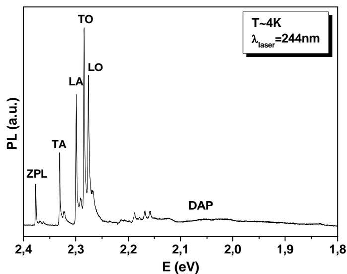
Fig. 2: LTPL spectrum collected at 4K on a high purity 3C-SiC VLS layer.
