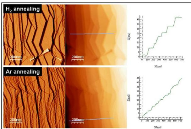
Fig.3: Effect of the thermal annealing performed on 4°off 3C-SiC(111) epilayer.
