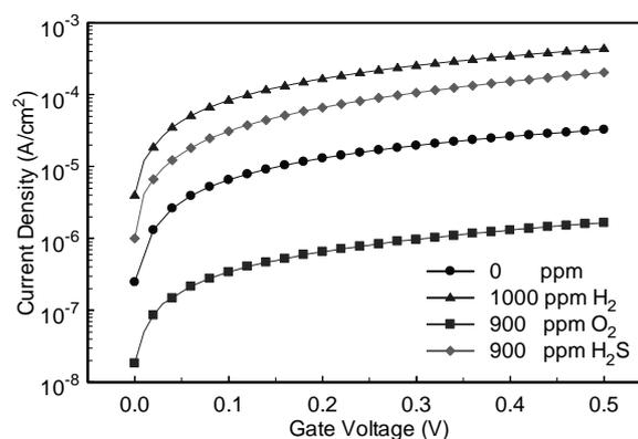
Fig. 2: Responses in different gases at 325°C.
