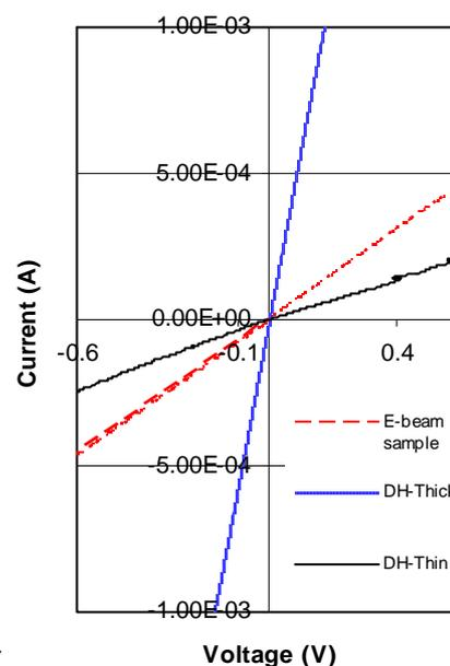
Fig. 2: Current versus voltage plot for the 4 points measurement, yielding the sheet resistance.
