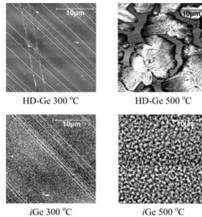
Fig 2: 25 $\mu$ m square AFM micrographs of the MBE Ge/SiC layers
