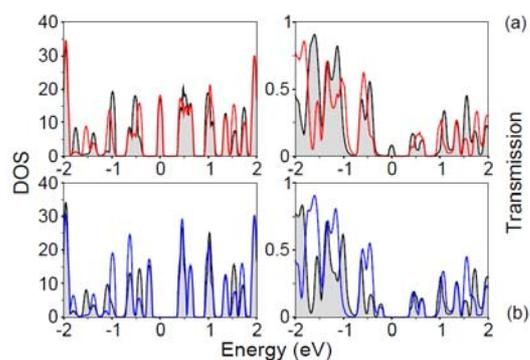
Fig. 3: Density of states and transmission probability by means of the Tight-Binding method for nonparameterized (a) and parameterized (b) vacancy values.
