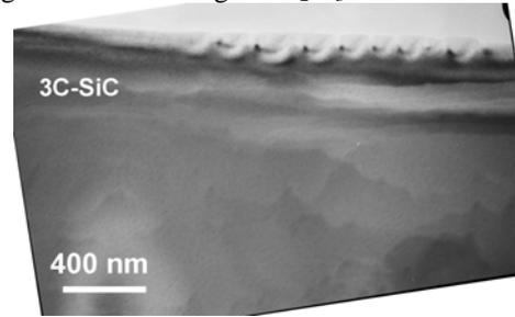
Fig. 3. A TEM image from the layer grown at temperature gradient 6 °C/mm. The 3C-SiC formed exhibits strongly reduced defect density.
