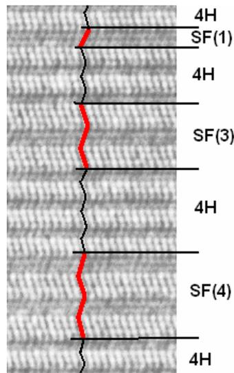
Fig. 2: Cross-sectionnal high resolution TEM image of various 3C-like zigzag faults in 4H-SiC. SF(1), SF(3) and SF(4) mean, respectively, 1, 3 and 4 zigzagged sequences of 3 bilayers of 3C.
