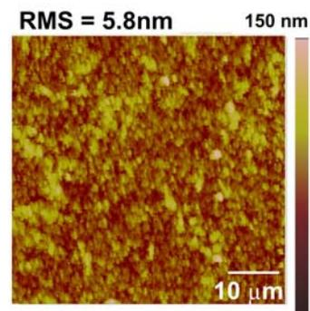
Fig. 3: AFM image showing surface topology of Si/SiC heterojunction structure.
