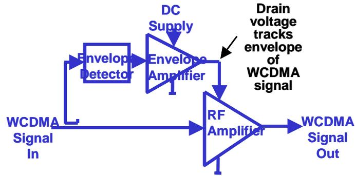
Fig.1: Schematic diagram of Envelope Tracking base station power amplifier.
