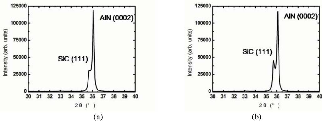
Fig. 3. XRD spectra of 3C-SiC films using (a) procedure I and (b) procedure II (synthesis temperature: 1200 °C, H<sub>2</sub>/MTS flow rate ratio at 100).
