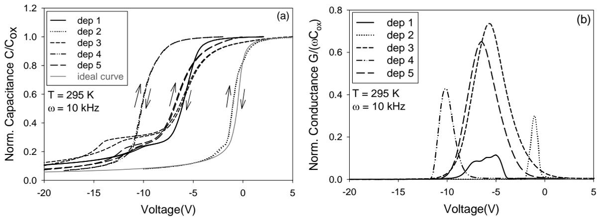
Fig. 1. Normalized C-V (a) and G-V (b) curves taken on 3C-SiC MOS capacitors fabricated by PECVD with post oxidation in N<sub>2</sub>O (1100°C), wet, and dry oxygen (950°C) for 3 hours (dep 1-3) or post annealed in N<sub>2</sub> at 950°C and 1100°C for 3 hours (dep 4 and 5).
