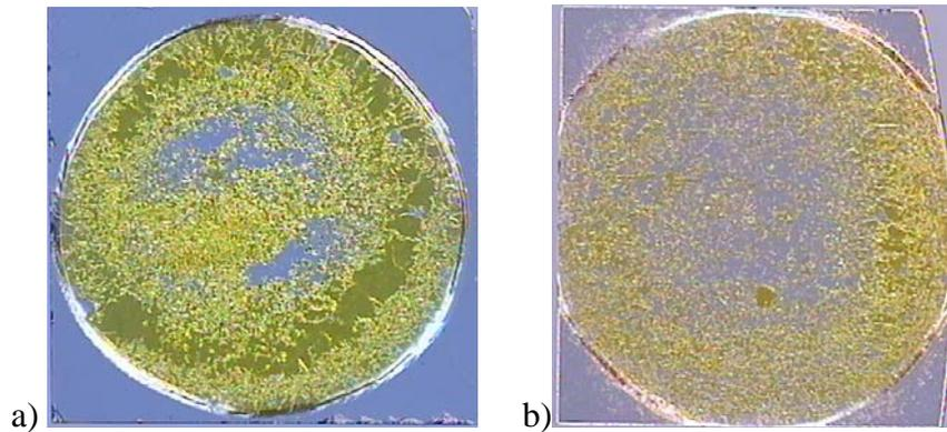
Fig. 1. (a) Image showing 87% of 3C-SiC in growth on as received substrates; (b) images showing 45% of 3C-SiC when using Si covered annealed substrates.
