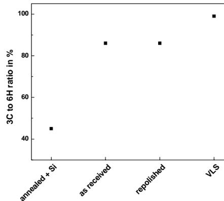
Fig. 2. Coverage of substrate by 3C-SiC in percent on differently prepared substrates.
