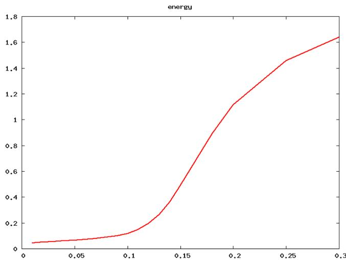
Fig. 1: Calculated average energy (eV) as function of the applied electric field (MV/cm) in bulk wurtzite GaN.
