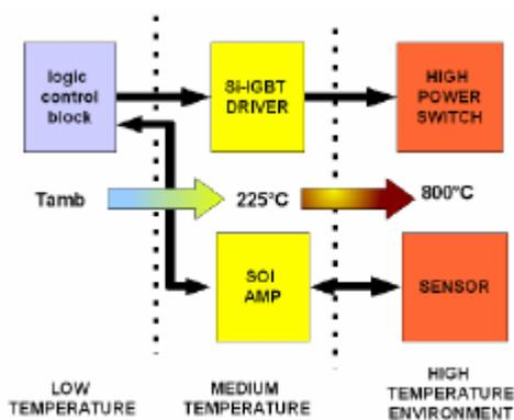
Fig 1: Usual "high temperature" converters topology using SOI technology for medium temperature range
