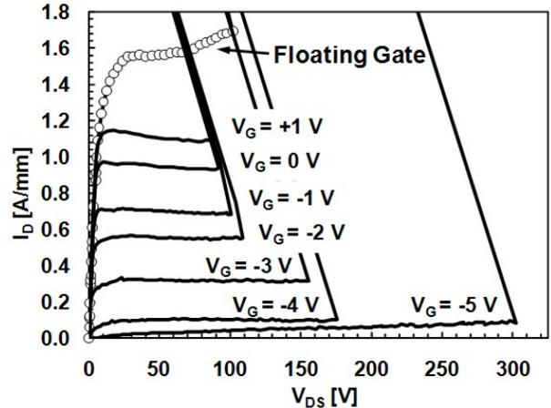
Fig. 4: I-V curves in 100 ns TLP regime to evaluate the breakdown points at different  $V_{GS}$ , and in floating gate condition ( $W = 800\mu\text{m}$ ,  $L_G = 0.5\mu\text{m}$ , SopSiC).
