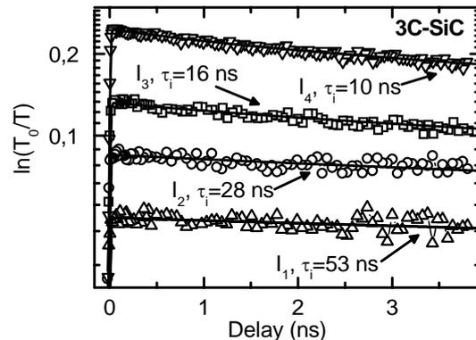
Fig. 2: FCA kinetics in bulk 3C-SiC at different excitations  $I$  ( $I_1$ - $I_4$  correspond to 6.6, 14.7, 24.4, and  $33.0 \text{ mJ}/\text{cm}^2$ ): experimental data (points) and modelling (lines), which provided Auger coefficient value  $C \approx 2 \times 10^{-32} \text{ cm}^{-6} \text{ s}^{-1}$ .
