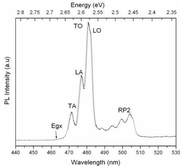
Fig. 1: LPTL spectrum collected at 5K on an in-grown stacking fault in a 4H-SiC epitaxial layer. One phonon (TA, LA, LO, TO) and two-phonon assisted recombination lines (RP2) manifest. The optical SF signature is  $\sim 2.672$  eV.
