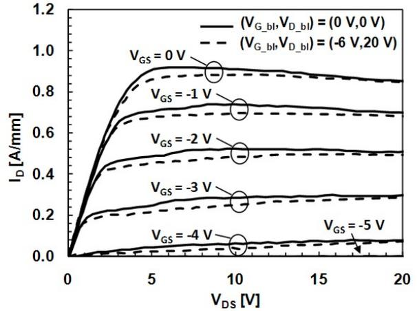
Fig. 2: DIVA-like measurements performed at two different quiescent bias points ( $W = 100\mu\text{m}$ ,  $L_G=0.5\mu\text{m}$ , SopSiC). Pulse width/Period=1  $\mu\text{s}/100\mu\text{s}$ .
