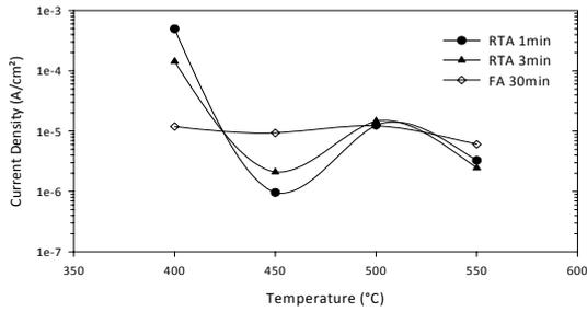
Fig. 2: Current density measured at 30V on non insulated "Schottky to Schottky structures" for different annealing durations, as a function of annealing temperature.
