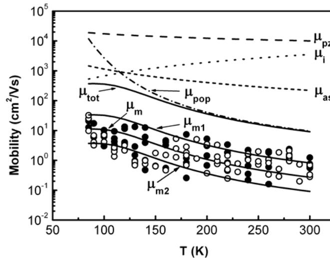
Fig. 2: Experimental and calculation hole mobility as a function of temperature for the *p*-type ZnO films
