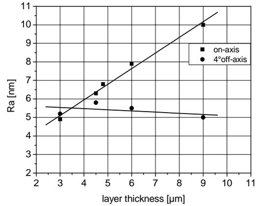
Fig. 3: Surface roughness Ra of 3C-SiC layers in dependence on layer thickness of on-axis and off-axis Si(001) substrates.
