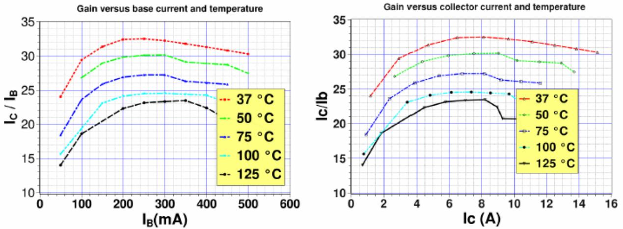
Fig 3: Current gain versus, base current (left), collector current (right), depending on temperature.
