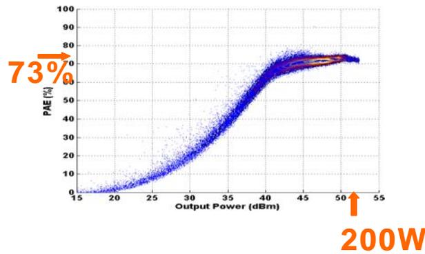
Fig.2: Instantaneous power-added efficiency vs output power for a GaN HFET measured during WCDMA operation in an ET amplifier.
