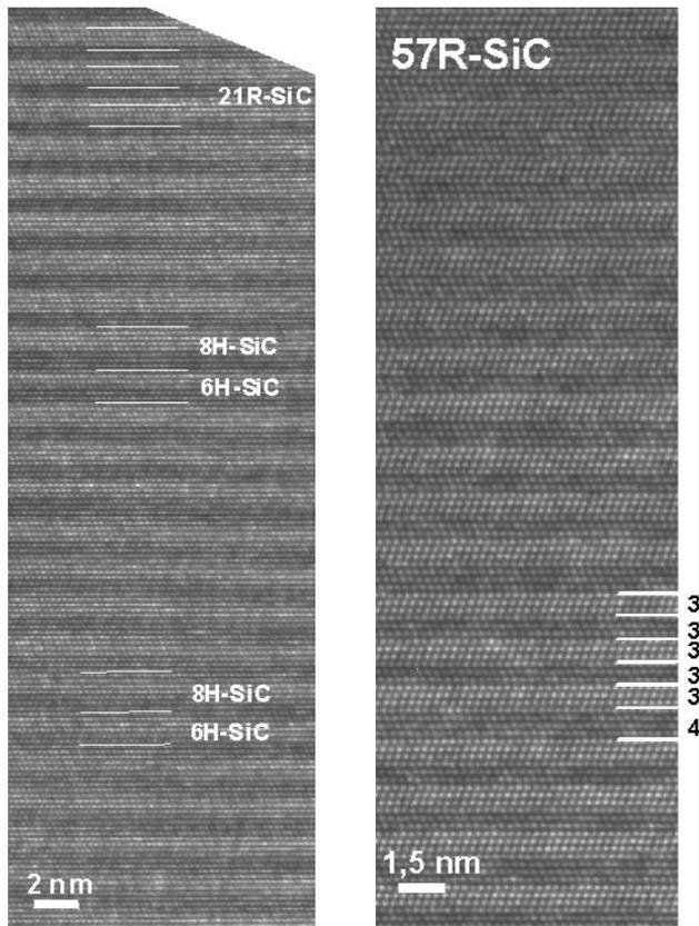
Fig. 2: HRTEM micrographs from (a) 21R-SiC showing the formation of SF induced lamellae of different polytypes; and (b) 57R-SiC.
