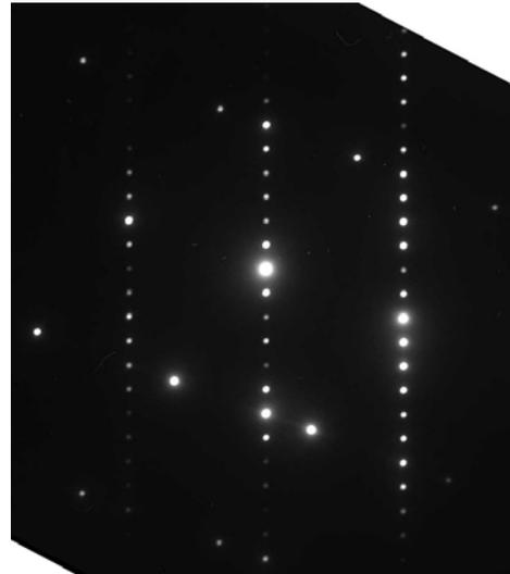
Fig. 4. A TEM image and the corresponding DP from the layer grown at the lowest temperature gradient 5 °C/mm, showing characteristic 3C-6H-SiC interface.
