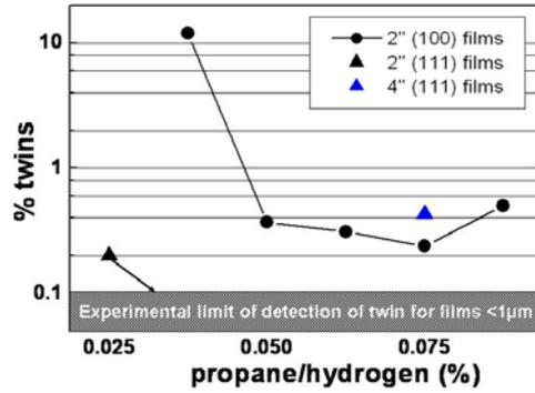
Fig.1: Evolution of the twin content within 3C-SiC epilayers grown on different substrates and for different propane dilution rates during the carbonization stage.
