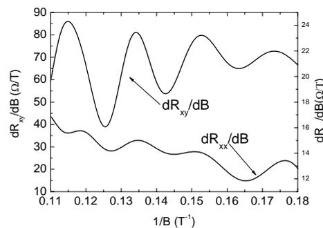
Fig. 1: Longitudinal magnetoresistance  $R_{xx}$  ( $d(R_{xx})/d(B)$ ) and transverse magnetoresistance  $R_{xy}$  ( $d(R_{xy})/d(B)$ ) in 3C/6H SiC heterostructures as a function of magnetic fields normal to the heterointerface at 1.5 K. as a function of  $1/B$ , after FFT smoothing.
