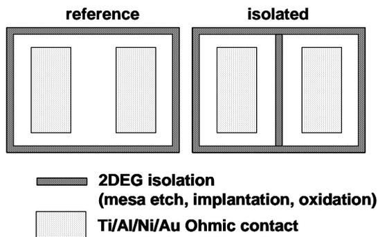
Fig. 1: Schematic of the structures used for testing the 2DEG isolation
