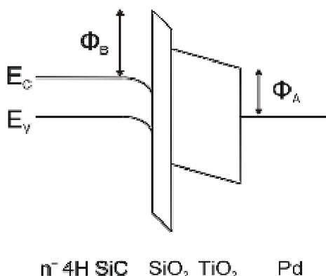
Fig. 3: Band diagram showing the barrier heights  $\phi_A$  and  $\phi_B$ .
