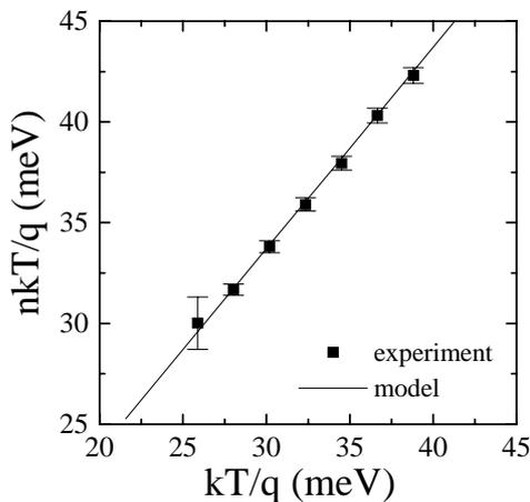
Fig. 1: Plot of  $nkT/q$  as a function of  $kT/q$  of macroscopic Au/Pt/GaN Schottky diodes and the theoretical curve obtained from the nanoscale barrier height distribution.
