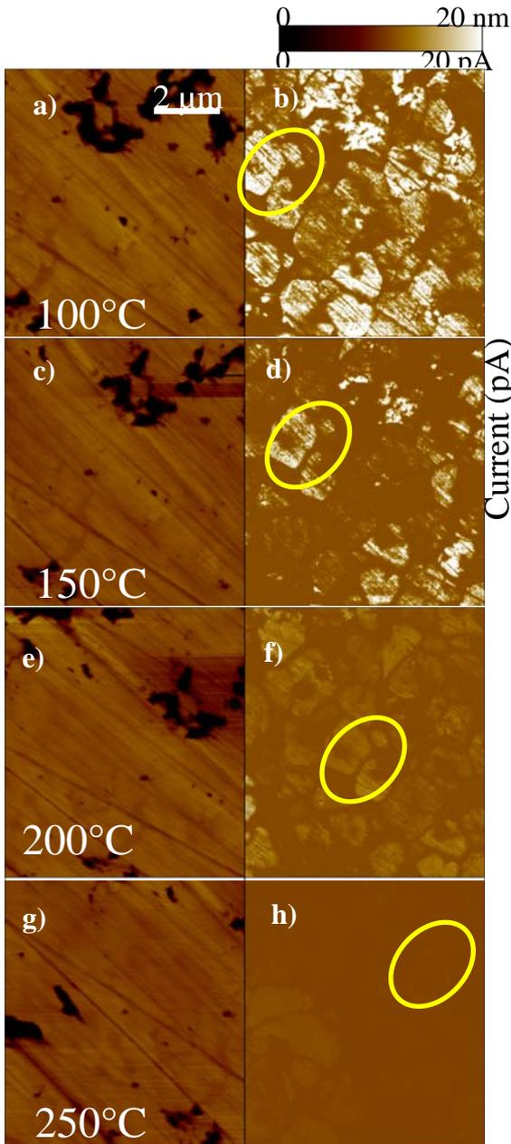
Fig.: 2: a), c), e), g) AFM morphology images. b), d), f), h) Current map acquired at 4 V at 100°, 150°, 200° and 250° C respectively.
