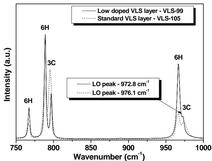
Fig. 1: Raman spectra of 3C-SiC layers grown by VLS using standard (red) and optimized (black) procedures
