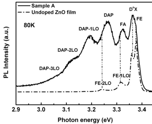
Fig. 1: PL spectra of undoped ZnO and N-doped *p*-type ZnO (sample A) at 80 K
