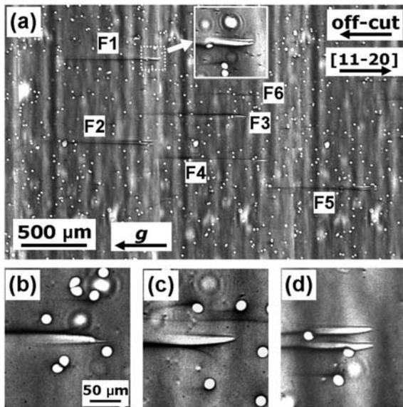
Fig. 5: Back reflection image recorded from a 4H-SiC epilayer showing TSDs and various combinations of Frank partials and Frank faults (F1-F6) created by deflection of TSDs onto the basal plane at the epilayer interface.
