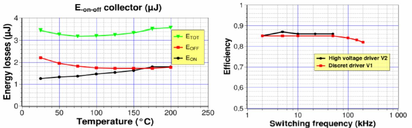
Fig. 7: Losses versus temperature (left), efficiency versus switching frequency (right).
