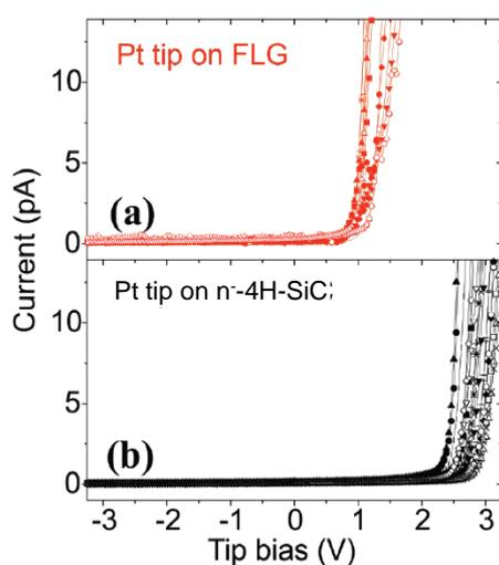
Fig. 2: An array of C-AFM carried out with a Pt coated Si tip measured (a) on few layer graphene (FLG) deposited on  $n^+4H$ -SiC and (b) on  $n^+4H$ -SiC.
