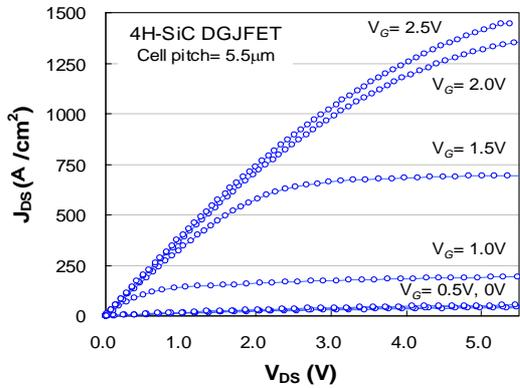
Fig. 5: Output characteristic of fabricated 5.5  $\mu\text{m}$  cell pitch normally-on 4H-SiC DGTJFET.
