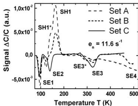
Fig. 2. Typical DLTS spectra of diodes with JTE (set A), diodes without termination extension (set B) and Schottky diodes (set C).
