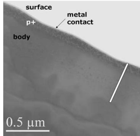
Fig. 2: TEM micrograph of Ti/Al bilayers deposited on Al ion-implanted 4H-SiC.
