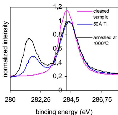
Fig. 1: C 1s peak of the XPS sample showing evolution of TiC after deposition of 50 Å Ti and subsequent annealing at 1000°C.
