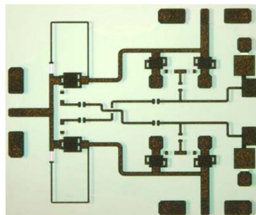
Fig. 5: Broadband Switch microphotograph
