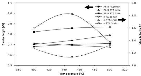
Fig. 4: Barrier heights (left-axis) and ideality factors (right-axis) for non lift-off SBD annealed 3min in RTA.
