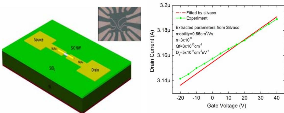
Fig. 1: (a) 3D device schematic view (inset: optical image of devices), b) experimental and fitted with Silvaco transfer characteristics of 3C-SiC NWFET
