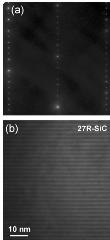
Fig. 3: (a) SADP revealing the formation of 27R-SiC (b) conventional XTEM image.
