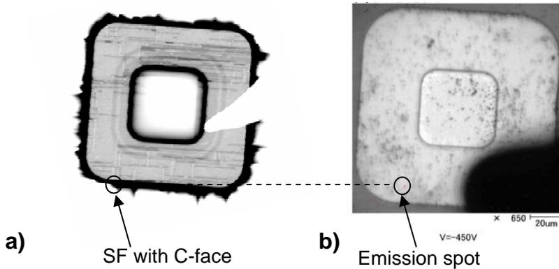
Fig. 3 a) EBIC and b) PEM image. A PEM spot located just on a SF which exposes C-face crossing the pn junction.
