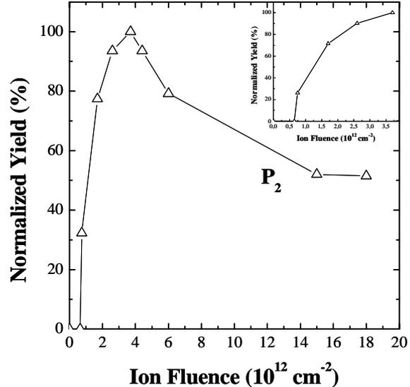
Fig 3: Normalised yield of  $P_2$  line group as a function of proton fluence. In the insert the low fluence range behaviour is shown.
