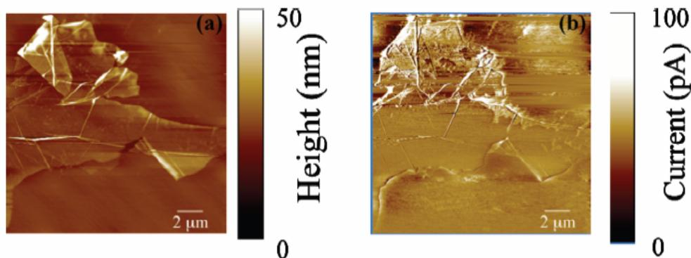
Fig. 4: Non destructive current mapping of graphene on SiC. Torsion AFM morphology is shown in (a), and the acquired corresponding current map on graphene in (b). The measured current amplitude depends on the underlying SiC surface morphology and the presence of graphene layers.
