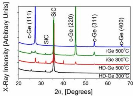
Fig 1: XRD  $\theta$ - $2\theta$  scans of the MBE Ge layers deposited on 4H-SiC
