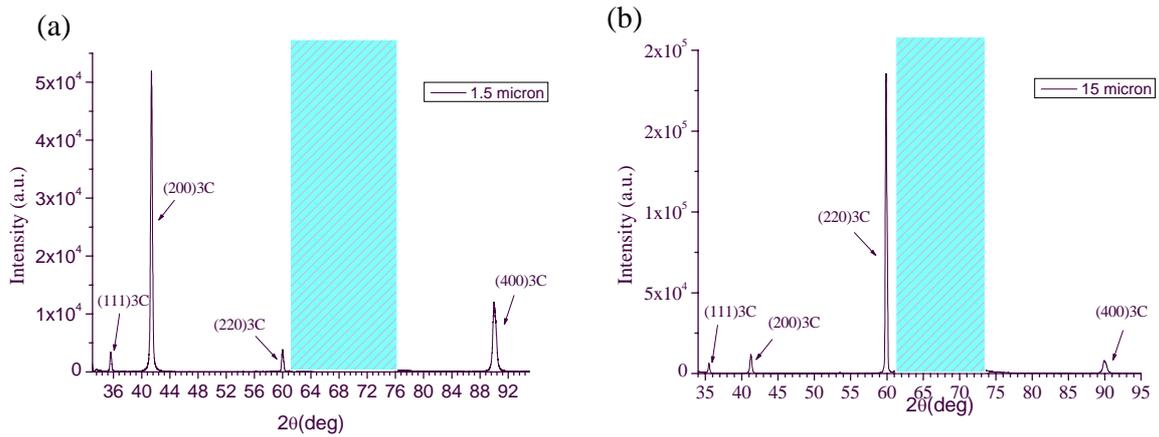
Fig.1: XRD patterns recorded in specular geometry ( $\theta/2\theta$  scan) for (a) a 1.5  $\mu\text{m}$  and (b) a 15  $\mu\text{m}$ , 3C-SiC film.
